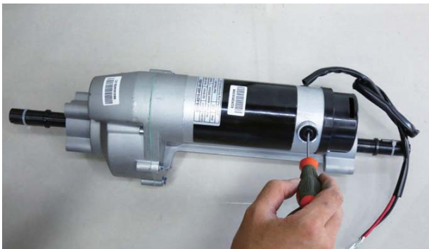
Figure 3 Disassembling the carbon brush of the drive motor
