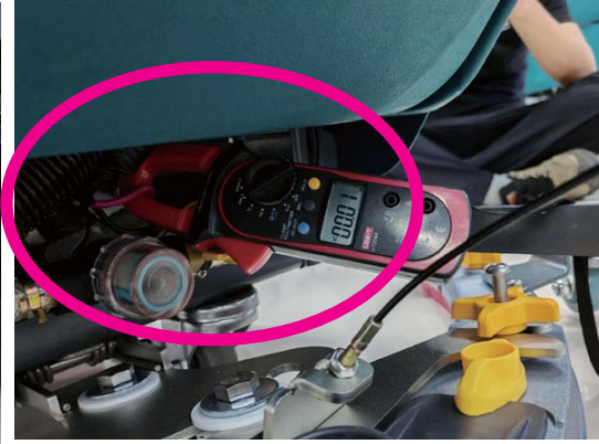
Figure 2 Measurement of no-load drive motor current
