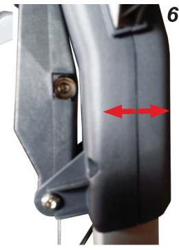
The microswitch mounted on the rear half-shell disables operation of the water pump when the front squeegee is activated. In the event of a pump malfunction, check the microswitch.
