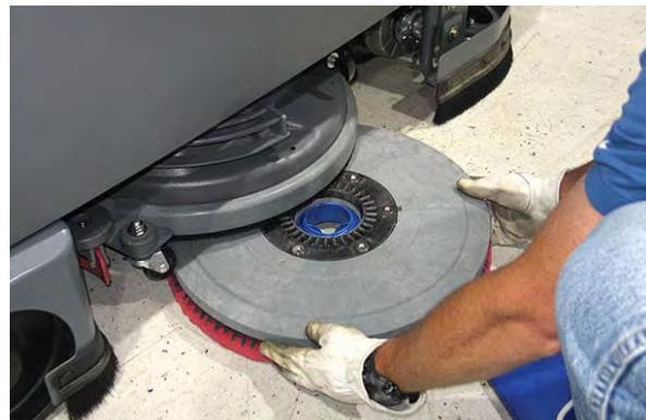
5. Push the new brush or pad driver under the scrub head and lift the brush or pad driver until the magnet secures the brush or pad to the drive hub.
