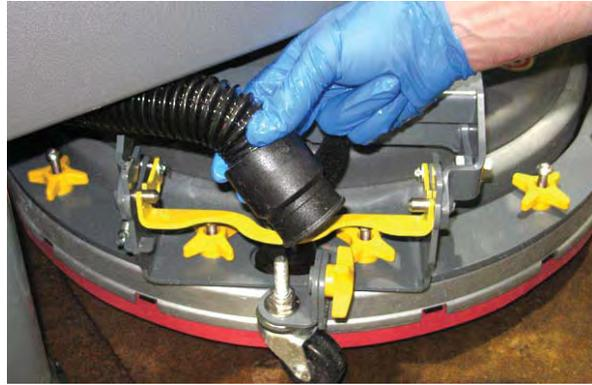
5. Squeeze the squeegee retainer lever and remove the squeegee assembly from the machine.
