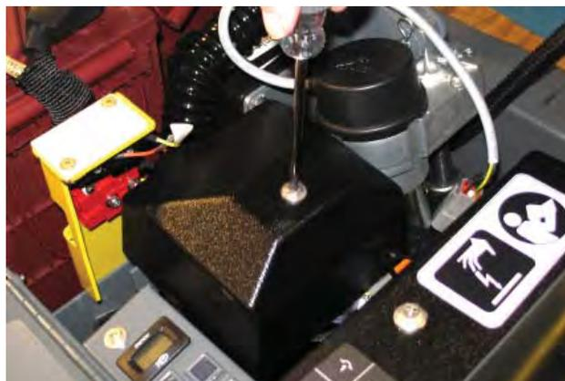
7. Disconnect wire harness connections from the top terminals of the contactor.
