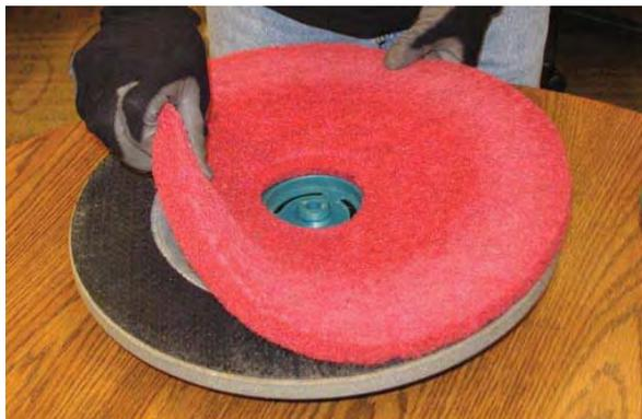
4. Reinsert the pad driver into the machine.
