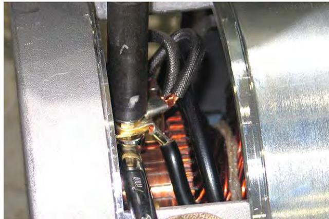
7. Push/lift the retainer spring from the carbon brush and remove the carbon brush from the scrub brush motor.
