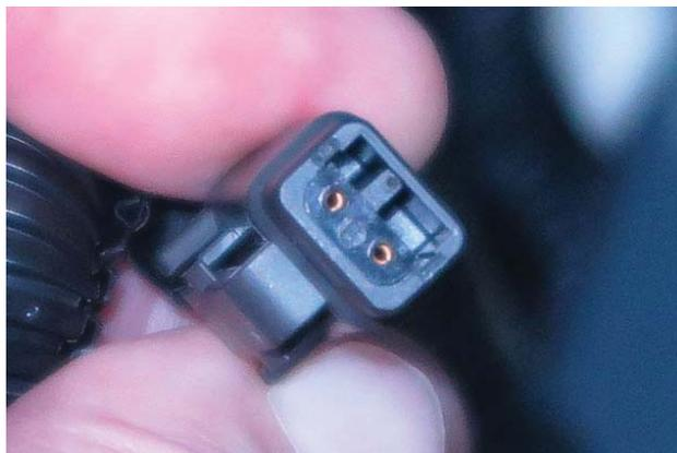
6. Inspect the resistor for damaged pins. Replace the resistor if pins are damaged/broken.
