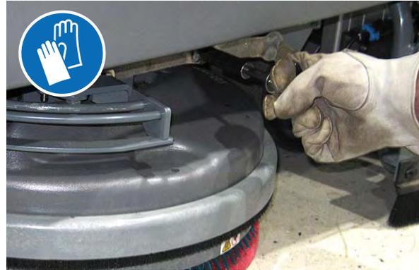
4. Remove the brush/pad driver from under the scrub head.
