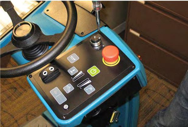
4. Carefully lift the control panel from the steering shroud. Do not break any wire or cable connections when lifting the control panel from the steering shroud.
