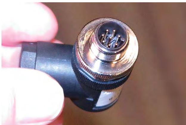
9. Check resistance between resistor plug pins 1 and 2 and pins 6 and 7. Resistance between pins 1 and 2 and pins 6 and 7 should be  $120\Omega$ . Replace the resistor plug if no resistance/excessive resistance.
