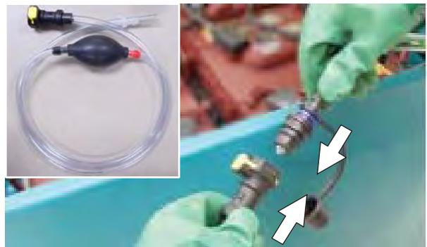
5. Submerge the other end of the hand pump hose into a bottle of distilled water
