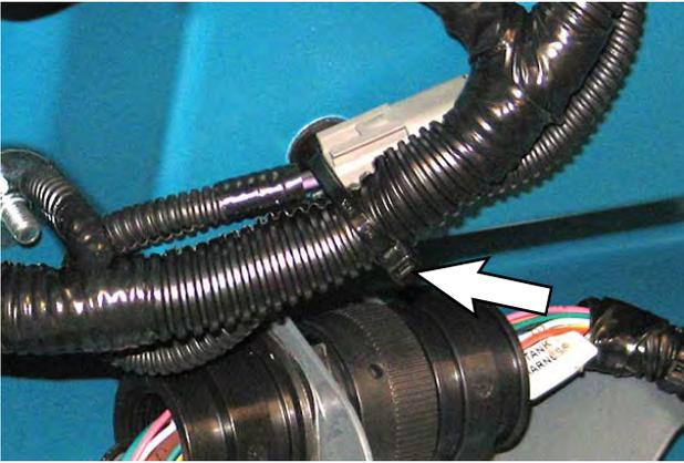
5. Disconnect the seat switch harness from the main wire harness.
