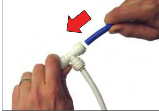
3. Push into the tube stop. The stainless steel teeth inside the collet firmly hold the tube in position and the o-ring provides a permanent leak-proof seal.
