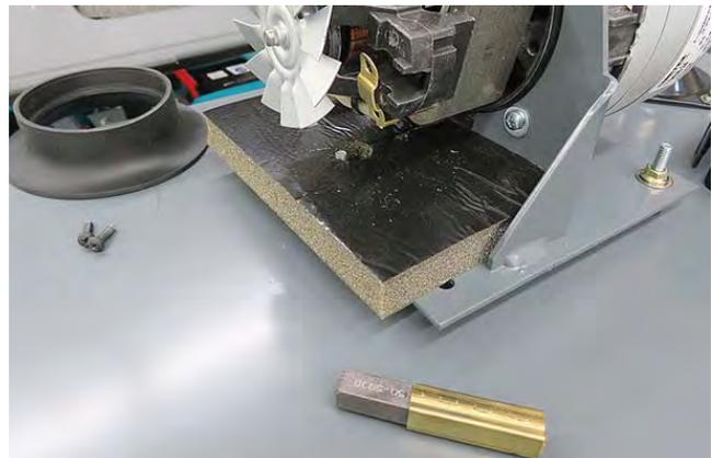
7. Inspect carbon brushes. Replace carbon brushes if they are stuck or are less than 10 mm (0.375 in.) in length.
