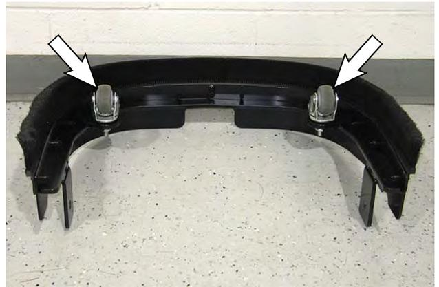
7. Install the caster wheels removed from the removed support bracket assembly onto the new support bracket assembly.
