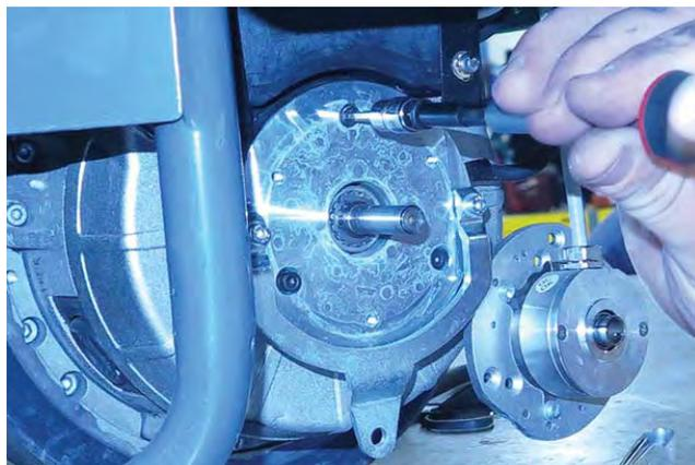
14. If replacing the brake assembly: Disconnect the wire harness from the brake assembly.
