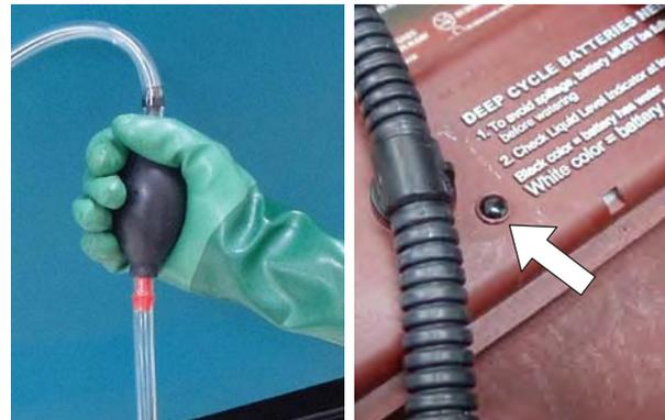
6. After adding water, replace the dust cap on the battery fill hose and store the hand pump hose inside the machine's battery compartment for future use.
