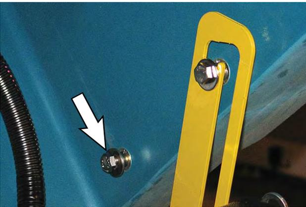
4. Use the hardware removed from the recovery tank in the previous step to secure the service cable to the recovery tank.
