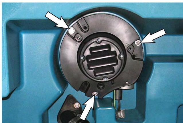
7. Remove the gasket from the vacuum fan.
