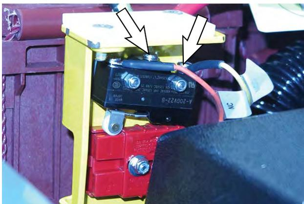
5. Remove the hardware securing the charger interlock snap switch to the connector bracket and the rear switch plate bracket.
