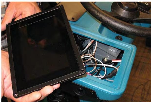
8. If replacing the touchscreen or if the touchscreen must be completely removed to service or replace other components, disconnect all wire and cable connections from the touchscreen and set the touchscreen aside somewhere where it cannot be damaged.
