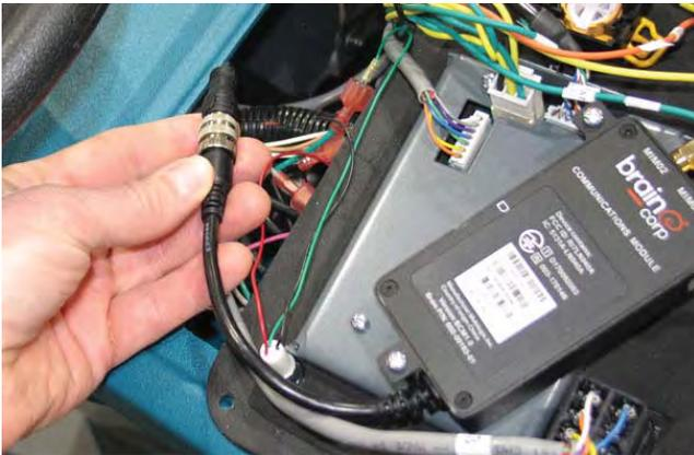
6. Remove the antenna/antenna bracket from inside the steering shroud.
