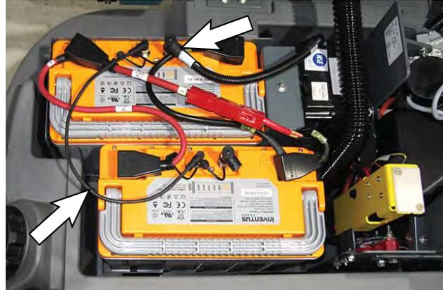
5. Repair/replace damaged lithium battery CAN communication cables. Ensure cables are all correctly torqued to the batteries.
