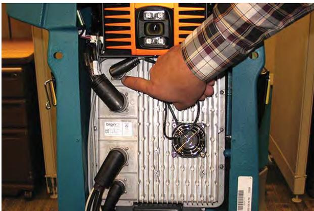
5. Cut all cable ties securing the touch screen cable to the machine.
