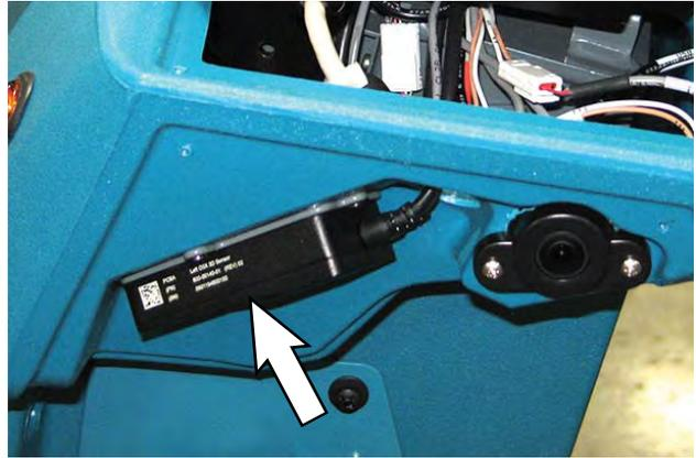
6. Disconnect the wire harness from the side 3D camera.
