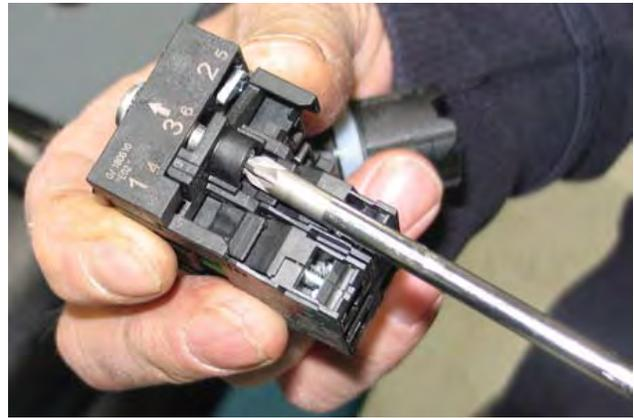
10. Install the new start/pause button assembly onto the start/pause button plate and tighten the retainer screw to secure the start/pause button assembly into place.
