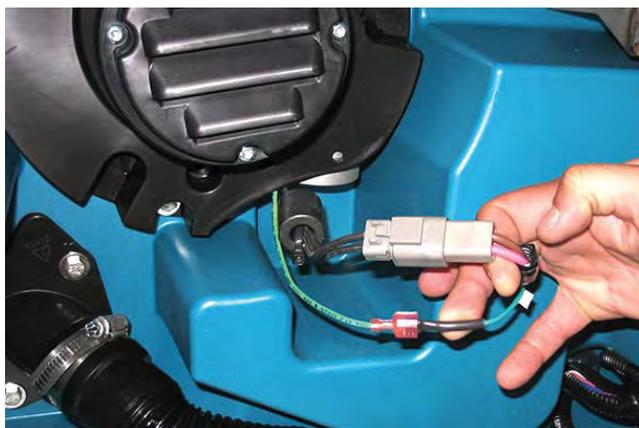
6. Remove the vacuum fan from the recovery tank .
