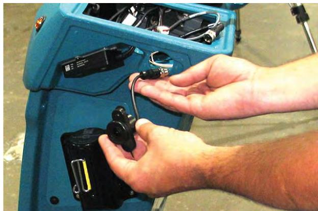
7. Install the new 2D camera into the steering shroud.
