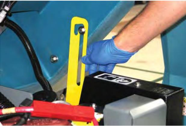
3. Remove the hardware for the service cable from the recovery tank.
