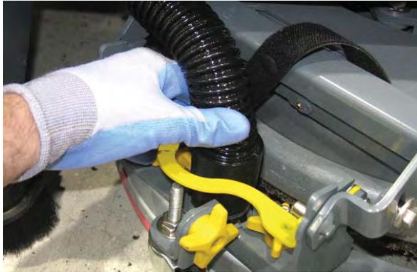
14. Use the hook-and-loop fastener to secure the vacuum hose to the squeegee assembly.
