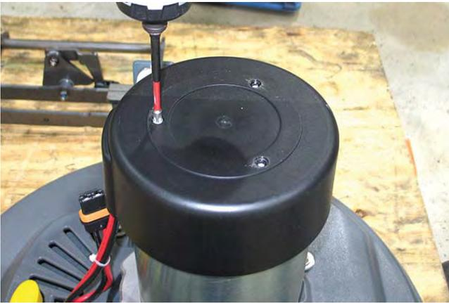
5. Remove the band from the scrub brush motor to access the scrub brush motor carbon brushes.
