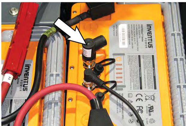
4. Check continuity between the corresponding pins at the lithium battery communication terminals (continuity is being measured across entire battery pack from the UI to BMS electrical harness communication terminal to the termination resistor communication terminal).
