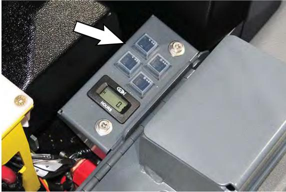
If the overload that caused the circuit breaker to trip is still there, the circuit breaker will continue to stop current flow until the problem is corrected.
