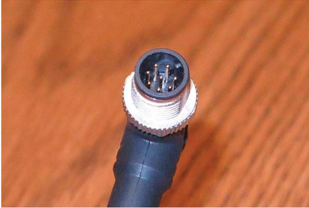
15. Check the resistance between the corresponding pins in the lithium battery CAN communication cable connectors on each end of each cable. Resistance between the corresponding pins should be 120Ω. Replace the cable if no resistance/excessive resistance.
