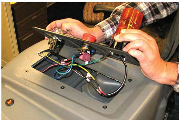
5. Disconnect the harness connections from the E-Stop button connector.
