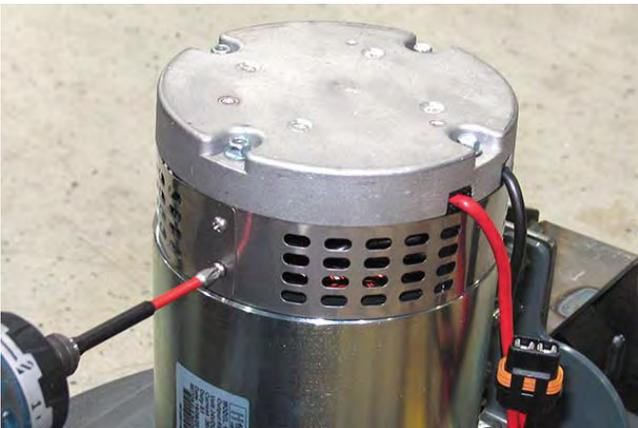
6. Remove the hardware securing the carbon brush cable to the scrub brush motor.
