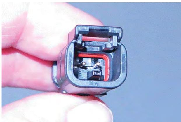
7. Check the resistance at the resistor pins. Should be 120Ω. Replace the resistor if no resistance/excessive resistance.
