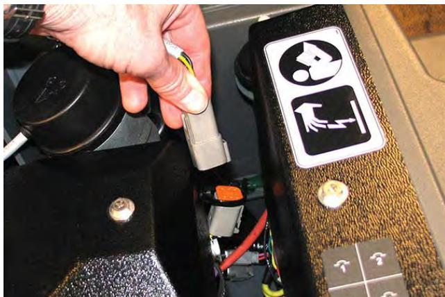
5. Remove the contactor cover from the contact mounting bracket to access the main contactor.
