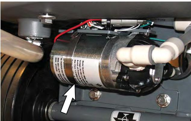
6. Disconnect both solution hoses from the *ec-H2O* pump.
