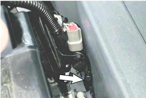
2. Attempt again to connect to the machine/access the lithium ion service screen. If issue persists, use another USB cable to connect the service device to the lithium battery control board USB cable.
