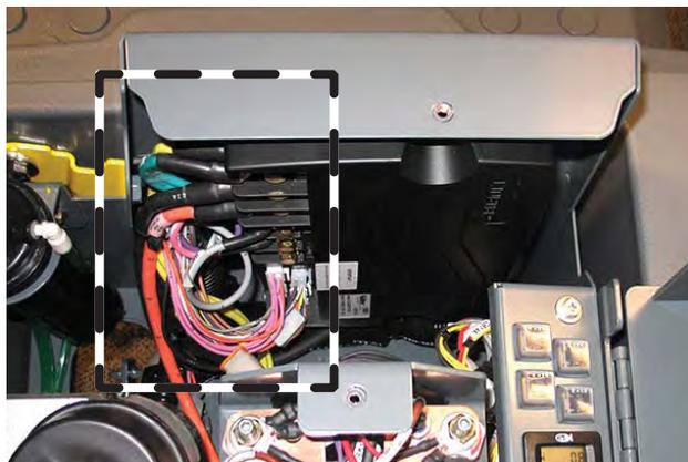
8. Remove the Kinetek controller from the machine.
