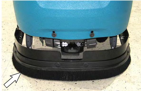
Inspect front perimeter guard adjustment plates located on both sides of the perimeter guard for slipping weekly. The entire top edge of the front perimeter guard must be parallel with the floor. Adjust the adjustment plates as necessary.
