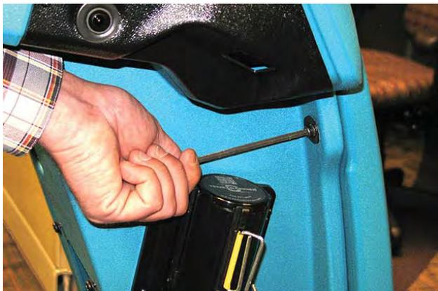
4. Remove the front shroud from the machine.
