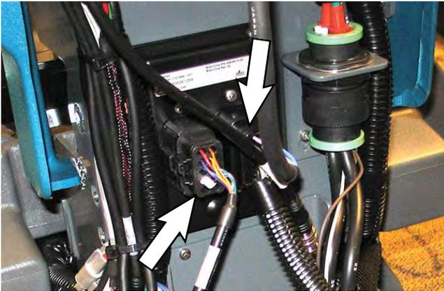
5. Remove the steering amplifier module from the steering column.
