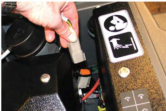
6. Remove the contactor cover from the contact mounting bracket to access the main contactor.
