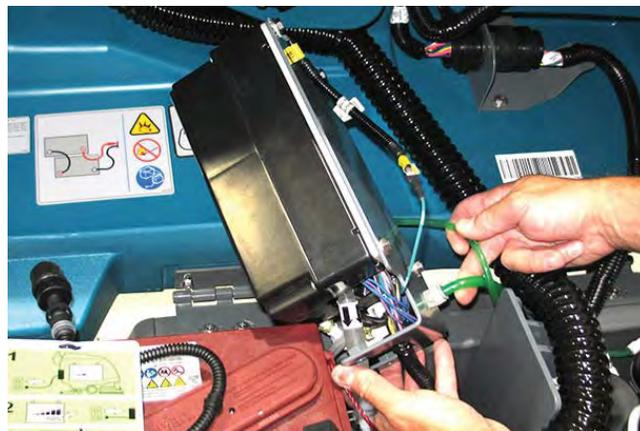
11. Remove the *ec-H2O* module from the *ec-H2O* mounting bracket.
