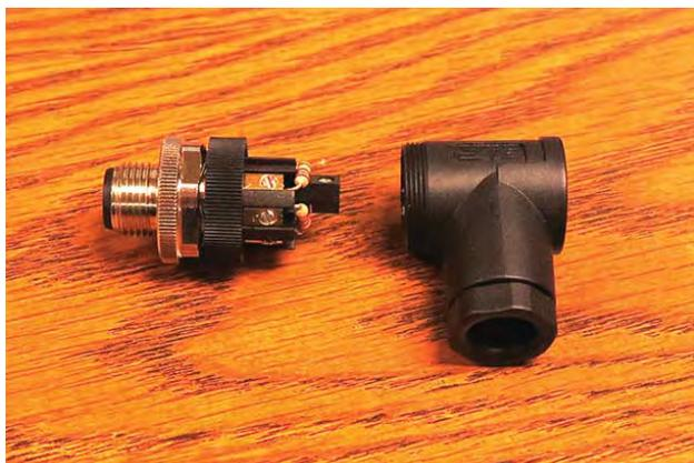
11. Inspect the resistor connections at the terminals inside the resistor plug. Both resistors should be undamaged and both ends of the resistors firmly secured inside the plug terminals.
