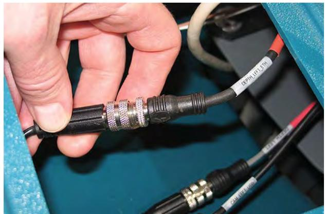
7. Remove the side 3D camera assembly from the machine.
