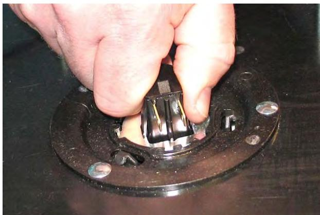
10. If replacing the seat switch, remove the adapter from the seat switch.
