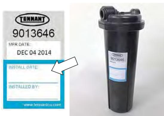
4. Install the new cartridge and reconnect the two hoses. Make sure the hose connectors are fully inserted into new cartridge.
