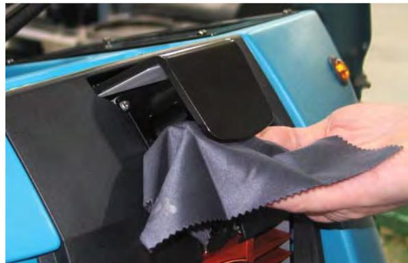
*NOTE: Due to the lower LIDAR sensor being located near the cleaning surface, pay particular attention to ensure the front, side, back, and bottom surfaces are completely clear of all dirt, smudges, and/or other debris. Use a flashlight to inspect these sensor surfaces and ensure they are thoroughly cleaned.*
