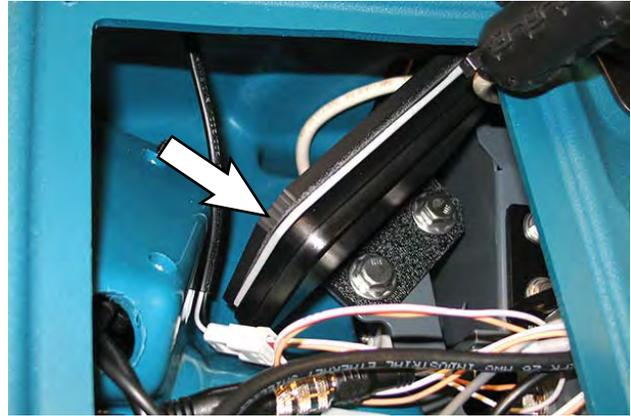
7. Remove the antenna from the antenna bracket.
