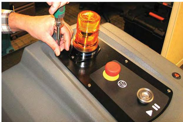
4. Carefully pull the rear control plate from the recovery tank cover. Do Not break or damage wire/cable connections when pulling the rear control plate from the recovery tank cover.
