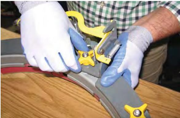
10. Align the squeegee carriage pins into the squeegee assembly bracket.
