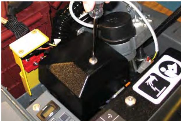
6. Remove the controller cover from the electric panel/machine controller.
