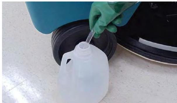
6. Squeeze the bulb on the hand pump hose until firm. The white float will rise when full.
