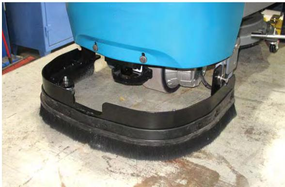
The jacking location at the front of the machine is located on the back of the LIDAR bracket. **Do Not** position the jack or jack stand at the front of the LIDAR bracket.
