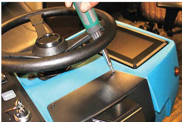
4. Remove the hardware securing the control bezel to the front of the instrument shroud.
