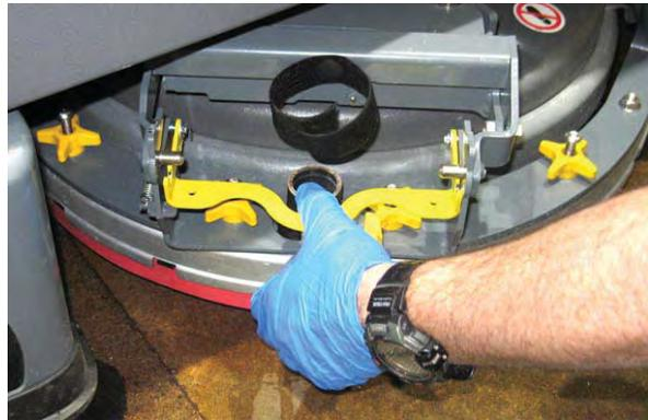
6. Fully loosen the four knobs on squeegee assembly. This will separate the spring loaded blade retainer from squeegee frame.
