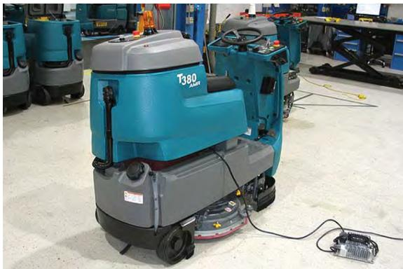
To engage the higher level, raise the recovery tank/seat and engage the recovery tank prop arm. This level also provides adequate space to perform maintenance to components located inside the battery compartment.
