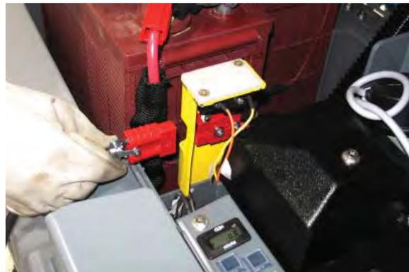
8. The charger will automatically begin charging and shut off when fully charged. The maximum charging cycle may take up to 6-12 hours depending on battery type.
