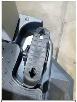
No brake pedal; acceleration and reverse is integrated
