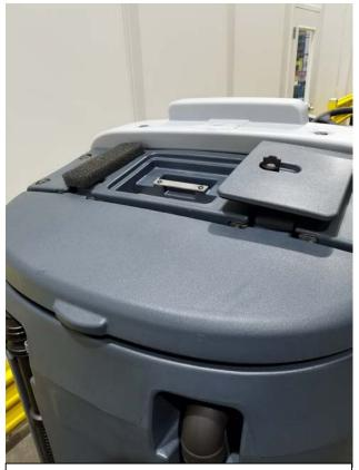
Vac fan filter and cover are not tethered to the machine – can be lost easily
