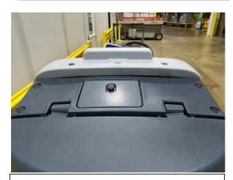
7 bolts on top of the machine plus more underneath; you have to remove the light and dark grey parts to access the vac fan
