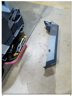
Side step is integrated in the side door. Side door is removal which can be lost and is difficult to put back on
