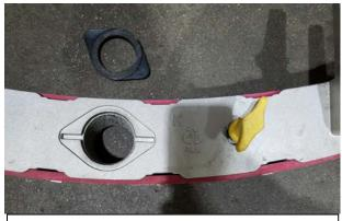
Removable gasket, if lost, can create a gap in the vacuum. Gap in vacuum = non-optimal water pickup
