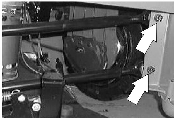
11. Pull the drag links out of the frame mount holes. Disconnect the kick-in guard from the front, right corner of the scrub head.
