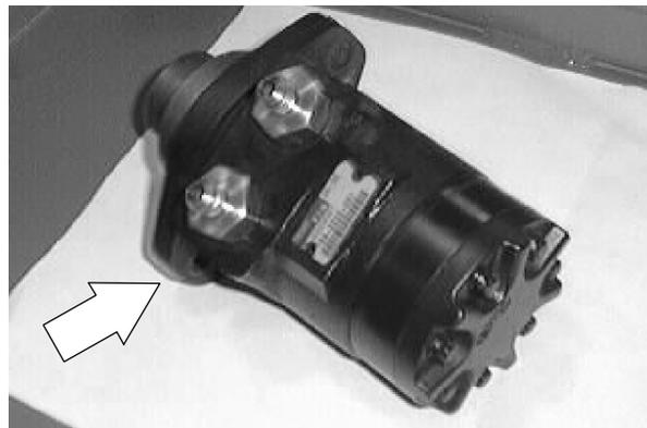
11. Remove the hydraulic fittings and taper lock hub from the existing motor. Install the fittings and hub on the new motor. *Position the top of hub even with the top of the motor shaft. Make sure the key is installed on the motor shaft.*
