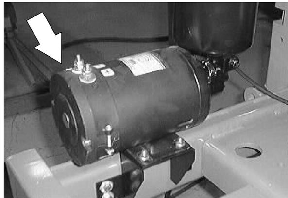
9. Reinstall the four M8 hex screws. Tighten to 18 - 24 Nm (15 - 20 ft lb).
