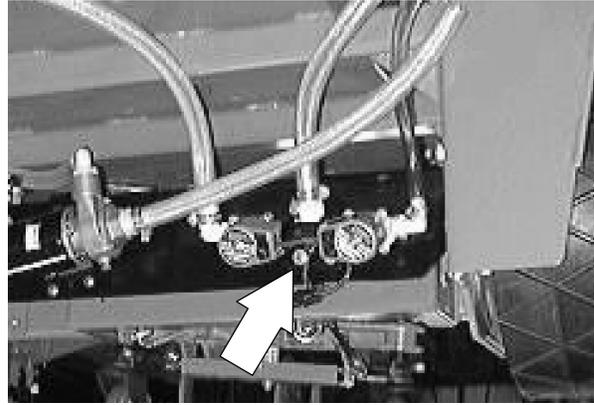
5. Disconnect the valve solenoids from the main harness.
