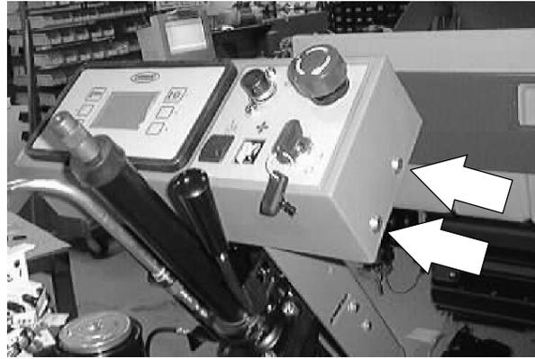
4. Remove the four wing nuts from the studs of the touch panel bezel.
