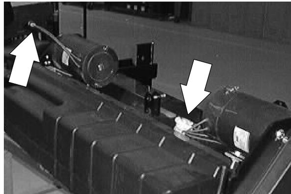
3. Remove the screws holding the plastic belt cover to the side of the scrub head. Remove the cover.
