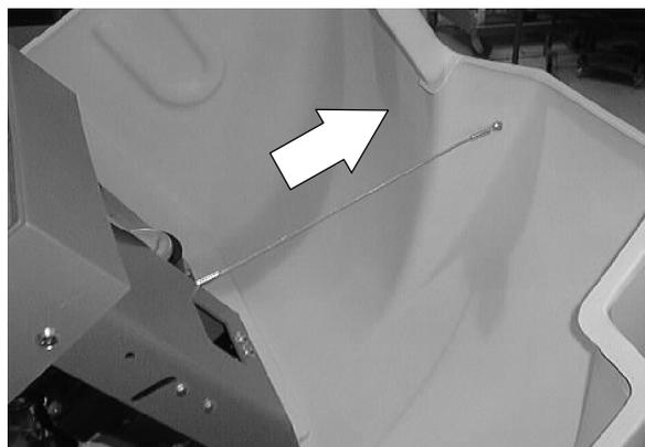
3. Remove the plastic traction motor cover.
