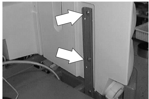
3. Loosely install the two hex screws holding battery cover mount plate to the inside of the solution tank.
