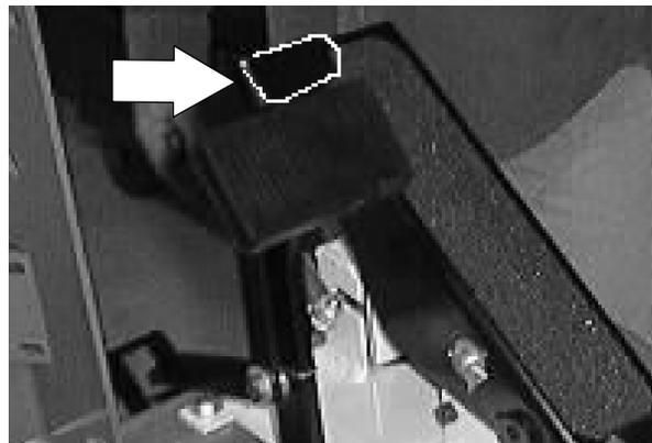
3. Open the side squeegee support guard with the latch. Swing the support guard outward to access the idler support casting.
