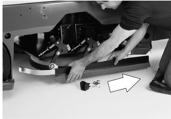
4. Install a new side squeegee blade onto the frame.
