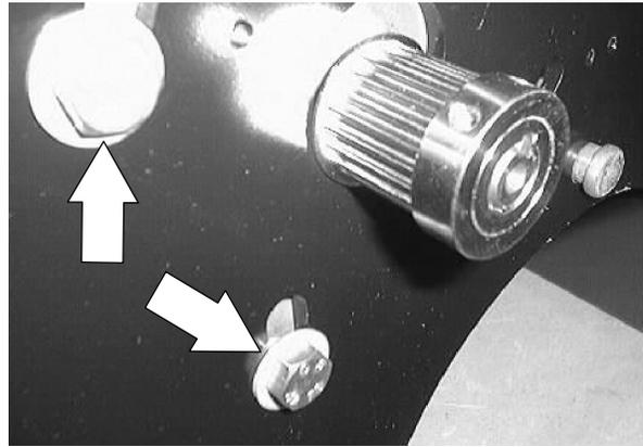
9. Loosen the allen screws holding the grooved pulley to the shaft of the scrub motor. Pull the pulley off the motor shaft. *Note the location of the pulley on the shaft.*
