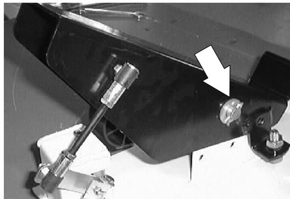
6. Remove the two pan screws holding the directional control unit to the mount bracket. Remove the unit from the mount bracket.
