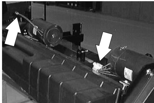
7. Disconnect the water flow solenoid from the main harness.
