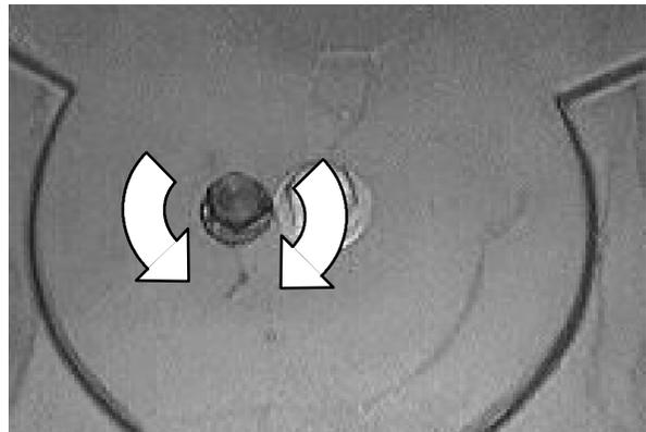
9. Check the brush patterns again and readjust as necessary until both patterns are the same.
