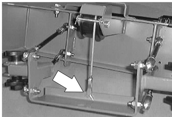
9. Operate the machine. Check the rear squeegee for proper operation.
