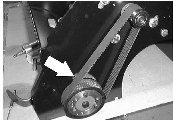
3. Remove the three hex screws holding the cogged drive sheave to the shaft hub.
