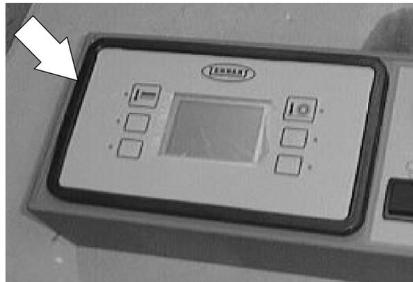
6. Remove the four screws holding the cover on the small control panel.
