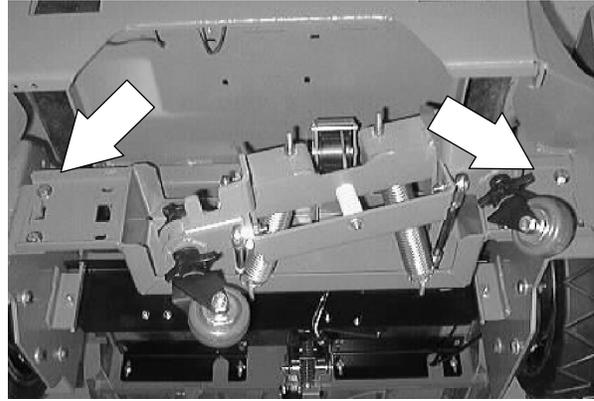
13. Reinstall the squeegee blade assembly frame onto the lift bracket. Position the vacuum hose into the hole in the squeegee frame.
