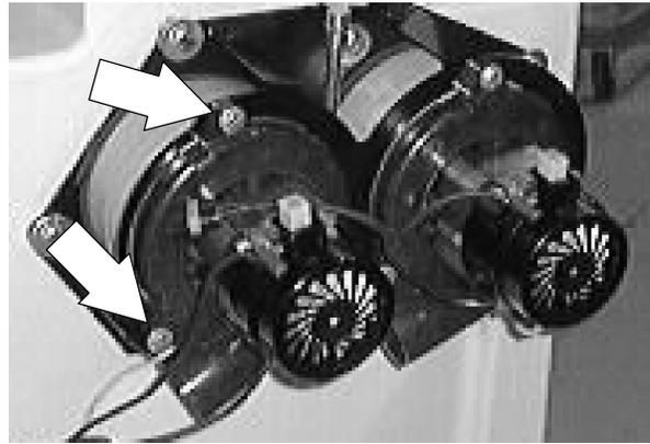
9. Reconnect the vacuum fan to the main electrical harness.
