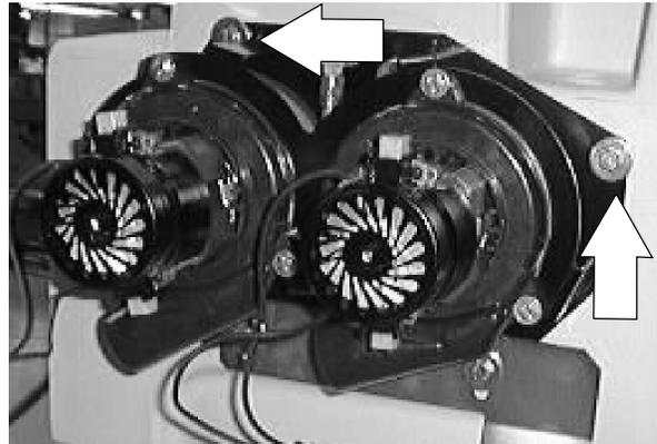
2. Reconnect the vacuum fan motors to the main harness.
