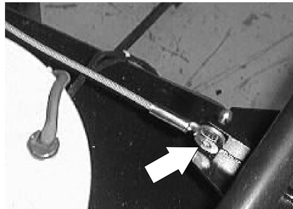
12. Reconnect the end of the side shift gas spring where it attaches to the scrub head. Reconnect the kick-in guard to the front, right corner of the scrub head.
