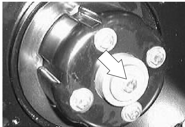
15. Reinstall the cogged sheave shaft hub onto the outside of the shaft and bearing assembly.
