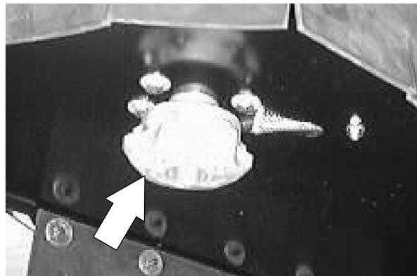
7. Push the scrub brush up until the spring clips lock onto the drive hub.
