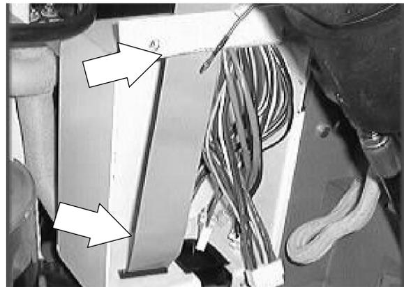
9. Pull the touch panel assembly back. Route the ribbon cable out of the grommet on the dash mount plate. Remove the touch panel and ribbon cable from the machine.
