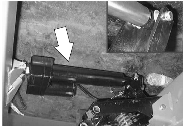
8. Reinstall the clevis pin and cotter pin into the actuator where it attaches to the machine frame (*battery compartment*).
