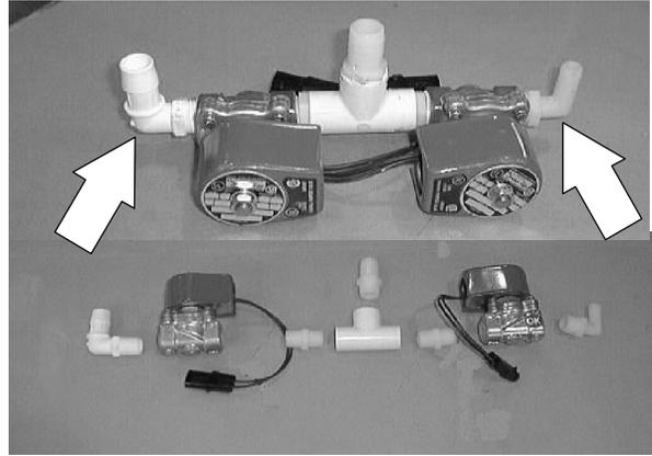
9. Remove the autofill valve from the plastic tee fitting.
