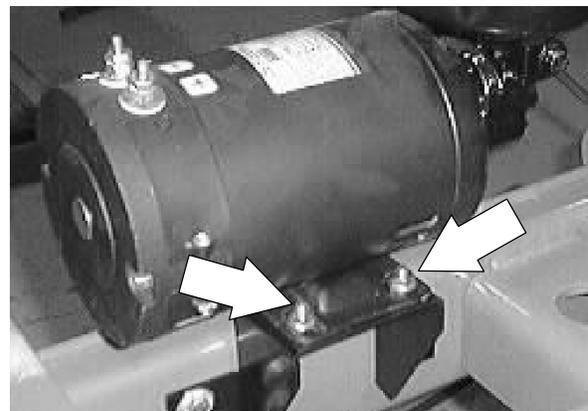
6. Remove the electro/hydraulic unit from the mount bracket.
