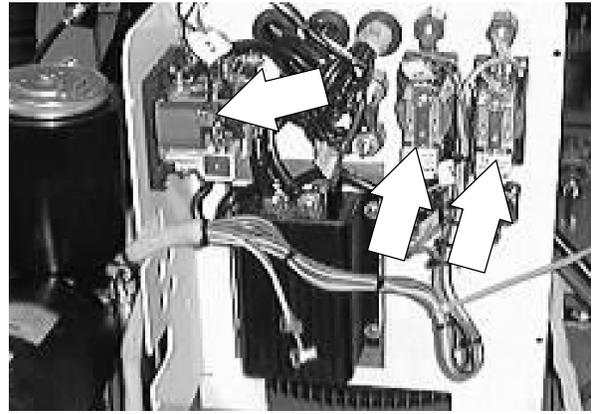
5. Mark and disconnect the electrical cables and smaller wires leading to the 36V relay.
