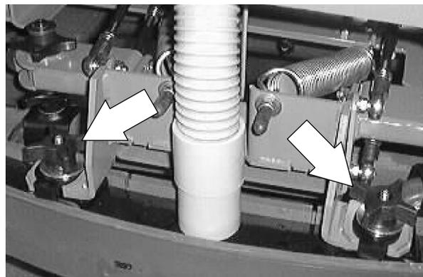
5. Operate the machine and check the squeegee assembly for proper operation.
