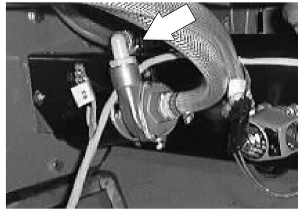
6. Remove the four hex screws holding the ES™ pump to the mount bracket. Remove the ES™ pump from the machine.
