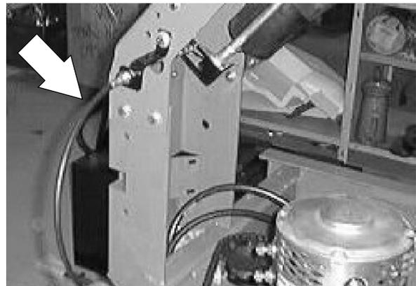
3. Loosen the large jam nuts holding the cable to the mount bracket. Move the cable in or out. Retighten the jam nuts.
