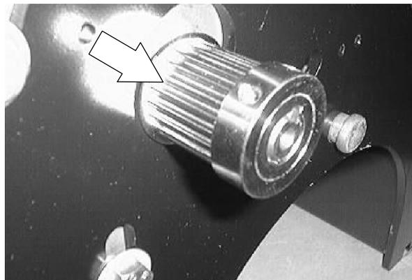
8. Finish removing the four hex screws holding the scrub brush motor to the scrub head. Remove the motor from the machine.
