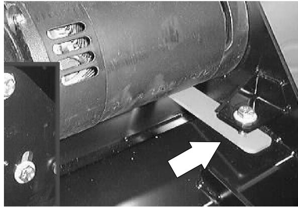
14. Go back and tighten the four brush motor screws to 37 - 48 Nm (26 - 34 ft lb).
