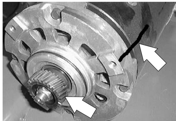
12. Position the traction motor back on the gear box housing. Make sure the electric cable studs are pointing towards the LH side of the machine.
