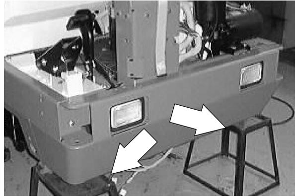
2. Push or pull the scrub head into the right side (operator's compartment side) of the machine. Push the head in until it is centered in the frame.
