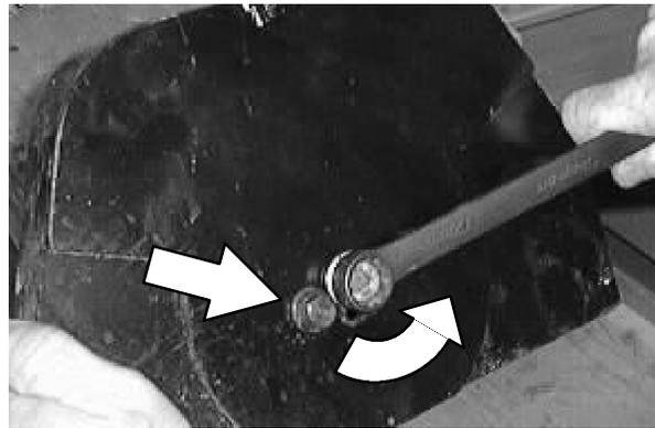
8. Using the smaller hex head - raise or lower the end of the brush as needed to straighten the brush pattern. Tighten the larger mounting screw.
