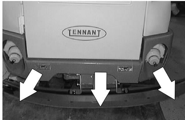
4. Loosen the large plastic jam nut located just above the squeegee caster on the side of the squeegee that needs adjusting.
