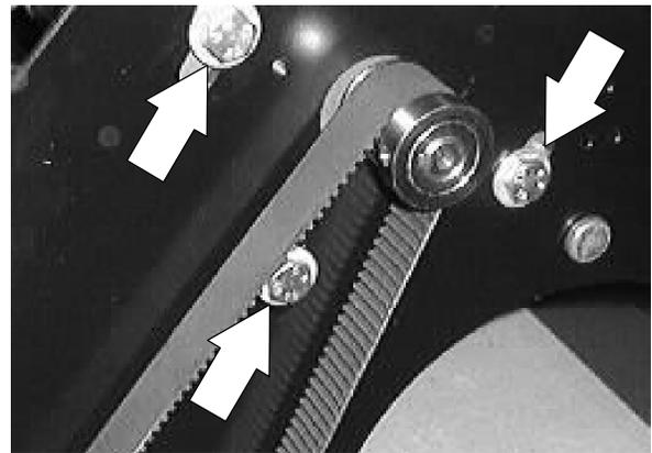
15. Check the alignment of the upper motor pulley with the lower drive pulley. Move the upper pulley in or out if needed.
