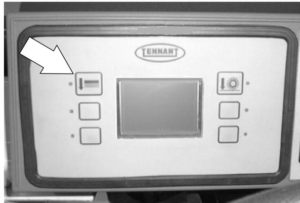
*NOTE: Use down pressure setting #3 on cylindrical head and down pressure setting #2 on all disc heads.*
