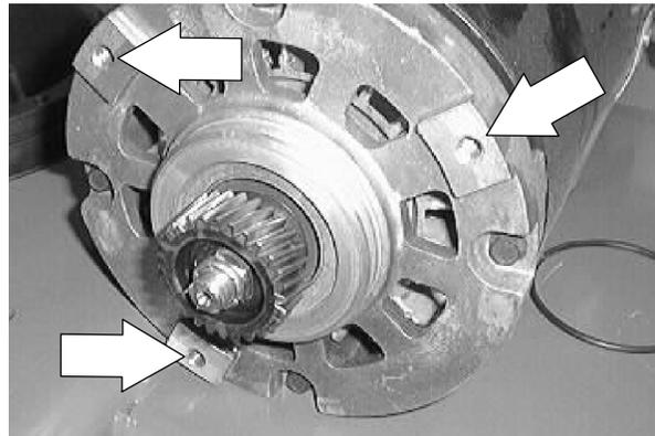
9. Pull the traction motor straight up and out of the drive gear box. Remove it from the machine.
