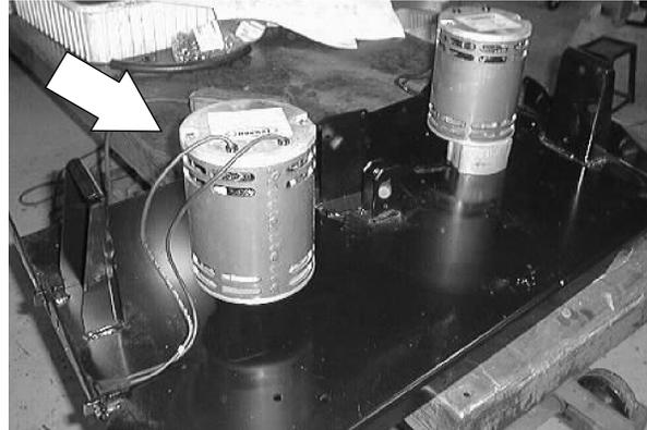
1. Turn on the machine and *lower* the scrub head. Shut off the key.
