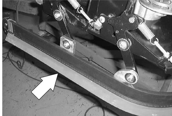
2. If the side squeegees need to have the down pressure adjusted--loosen the jam nuts on the tension spring threaded rod. Move the threaded rod down to increase tension on the spring. Retighten the jam nuts.
