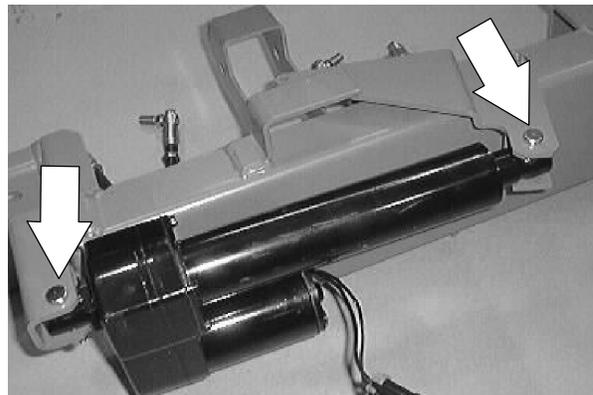
10. Position the squeegee assembly at the back of the machine. Reconnect the squeegee lift actuator to the main harness.
