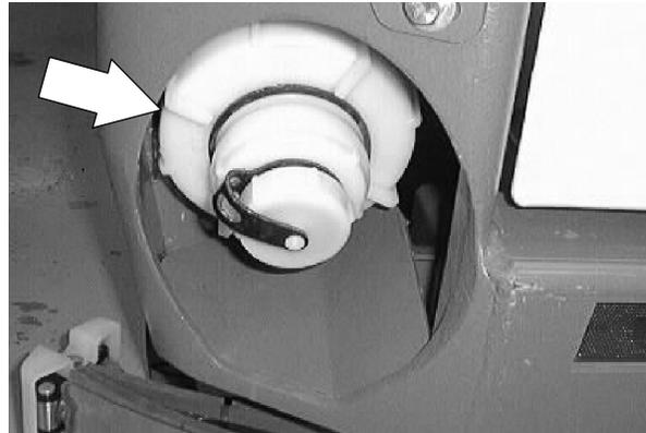
2. Go under the machine on the right side and locate the ES™ pump on the mount bracket between the back wheels.
