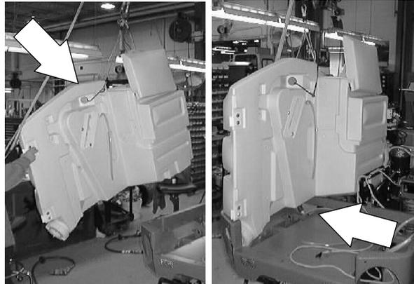
2. Loosely install the two hex screws holding the recovery tank to the vertical mount channel at the right side of the battery.
