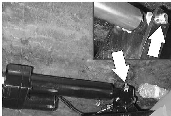
4. Go to the battery compartment and remove the cotter pin and clevis pin from the actuator where it attaches to the machine frame.
