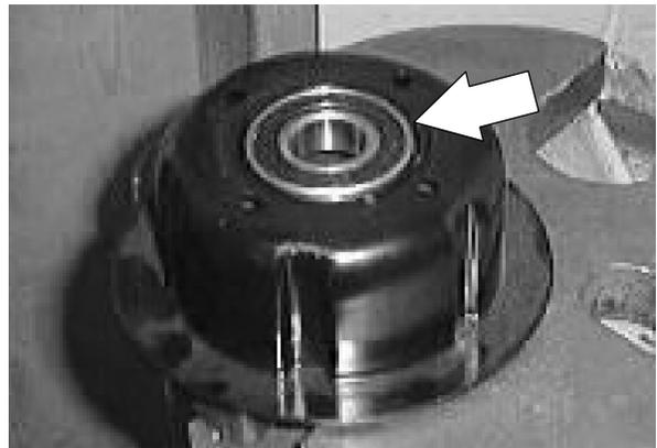
7. Use a mechanical arbor press to remove the existing bearing and to install the new bearing.
