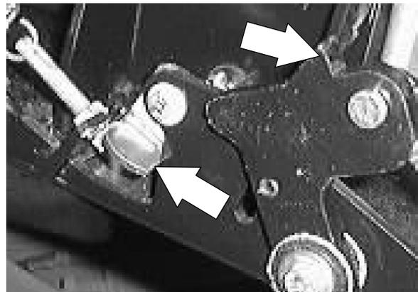
3. Reach into the scrub brush area and spin the scrub brush until the spring clips are visible.
