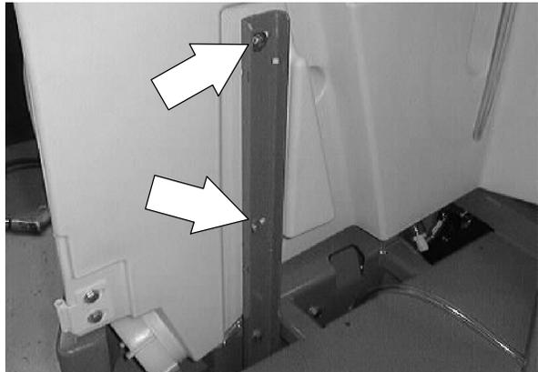
3. Reinstall the clamp holding the battery cables to the back of the recovery tank.
