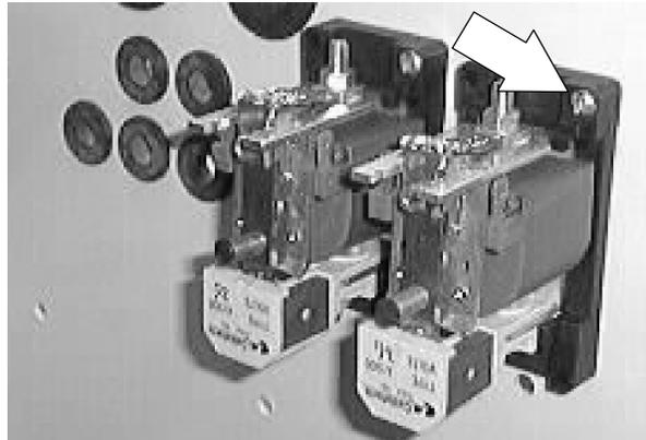
7. Install the new 36V relay onto the control panel. Reinstall the two hex screws. Hand tighten lightly--do not over tighten.
