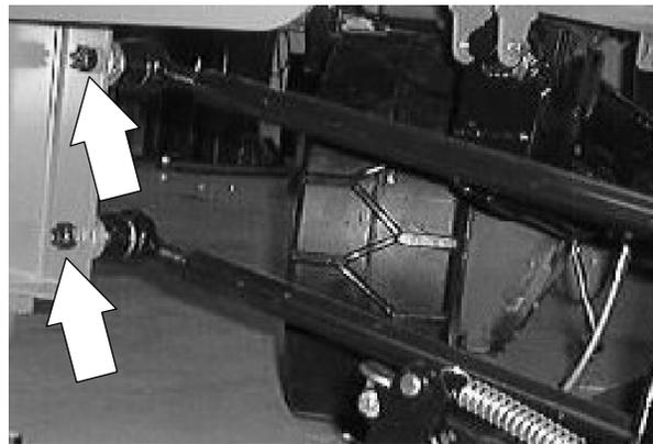
4. Reinstall the castle nuts onto the end of the scrub head drag links where they attach to the machine frame. Tighten the castle nuts tight. Reinstall the cotter pins.
