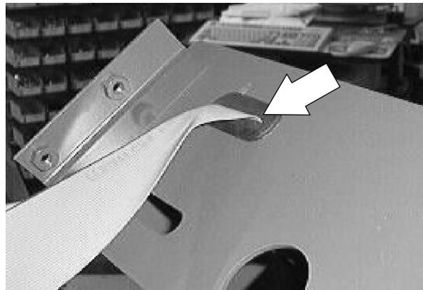
10. Install the new touch panel and ribbon assembly on the dash mount plate. Route the ribbon cable through the grommet and dash slot.
