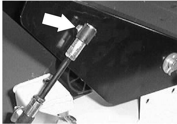
5. Remove the cotter pin from the large clevis pin holding the pedal to the directional control unit. Remove the pedal from the machine.
