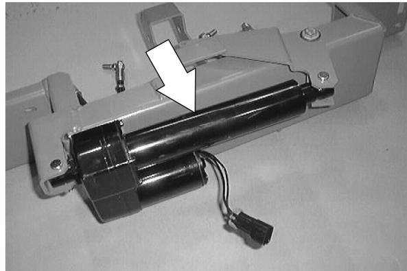
9. Reinstall the clevis pins and cotter pins into each end of the new actuator.
