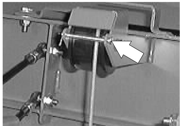
7. Reattach the squeegee lift cable to the actuator pivot bracket using the clevis pin and cotter pin.
