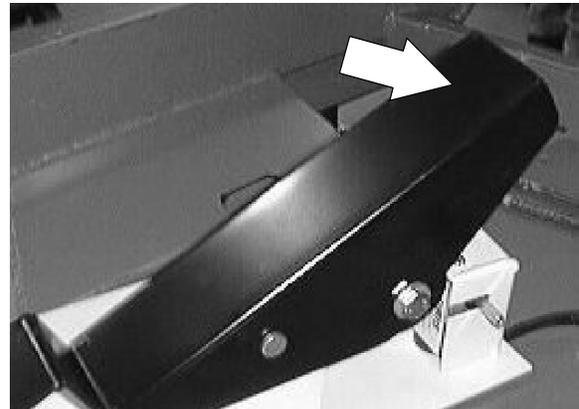
**Reverse:** Press the bottom of the directional pedal with the heel of your foot.
