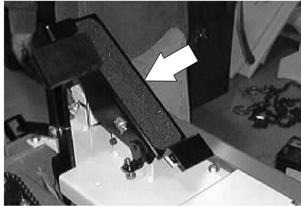
**Forward:** Press the top of the directional pedal with the toe of your foot.
