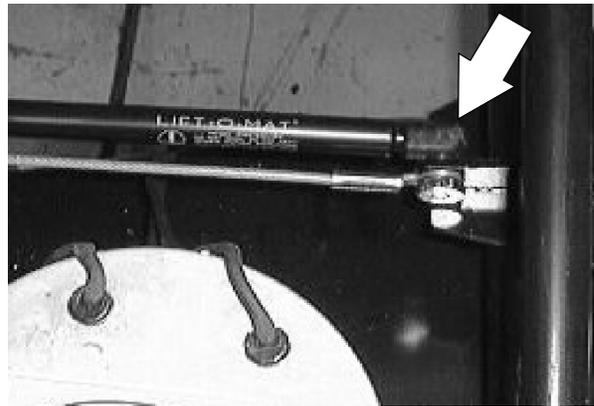
9. Disconnect the end of the side shift cable where it attaches to the scrub head.
