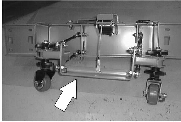
5. Disconnect the squeegee lift actuator from the main harness. The squeegee assembly can now be removed from the machine.
