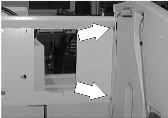
9. Remove the two hex screws holding the solution tank to the vertical mount channel at the right side of the battery.
