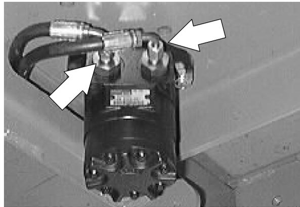
14. Reinstall the small steering chain sprocket onto the motor hub. Install the three hex screws. Leave loose for now. *Use loctite blue 242 on the threads.*
