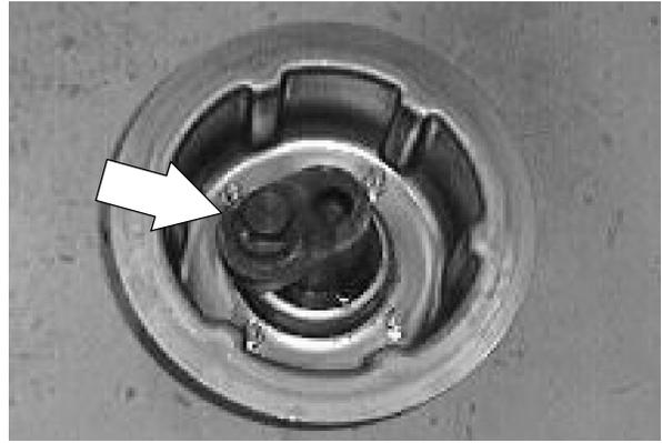
5. Remove the four screws holding the bearing retainer plate to the idler hub.
