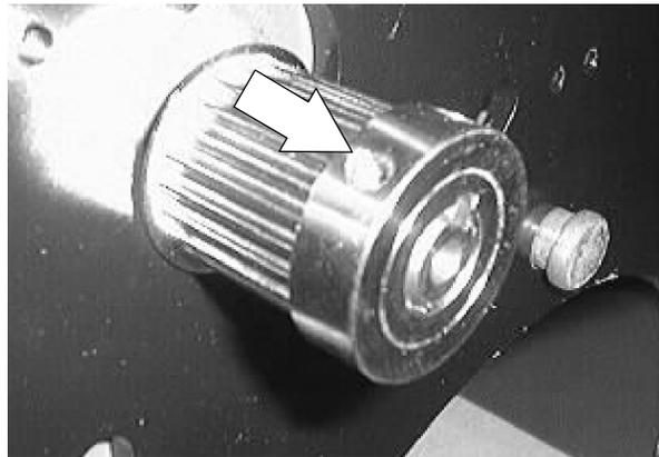
10. Install the grooved pulley onto the new scrub brush motor.
