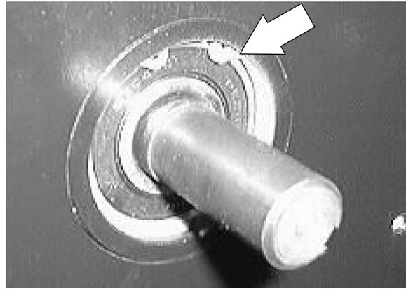
14. Reinstall the scrub brush drive hub onto the shaft on the inside of the shaft. Reinstall the hex screw and tighten to 8 - 10 Nm (5 - 7 ft lb).
