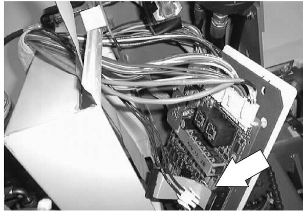
8. Route the ribbon cable out of the small control panel.
