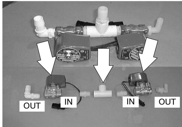
10. If replacing left hand autofill valve--note orientation of valve and fittings.
