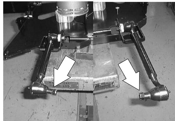
4. Reinstall the castle nuts onto the end of the scrub head drag links where they attach to the machine frame. Tighten the castle nuts tight. Reinstall the cotter pins.
