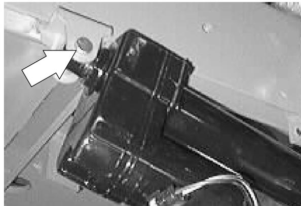
7. Position the new actuator in the machine. Reinstall the two clevis pins and cotter pins.
