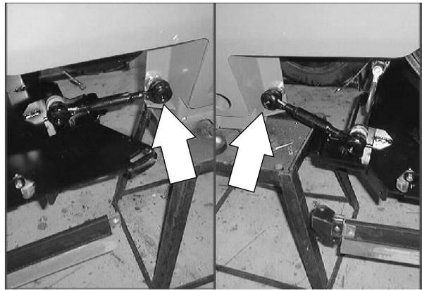
11. Pull the drag links out of the frame mount holes. Disconnect the kick-in guard from the front, right corner of the scrub head.
