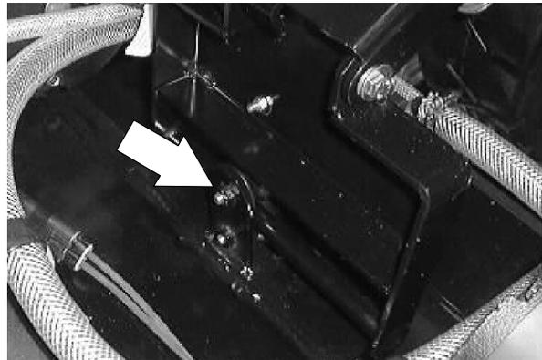
12. Reconnect the end of the side shift cable where it attaches to the scrub head.
