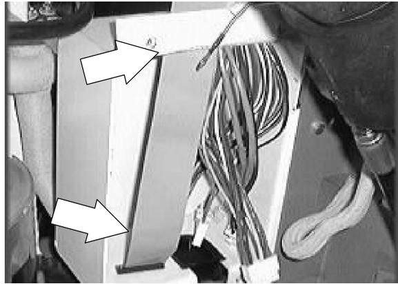
12. Plug the ribbon cable into the circuit board.
