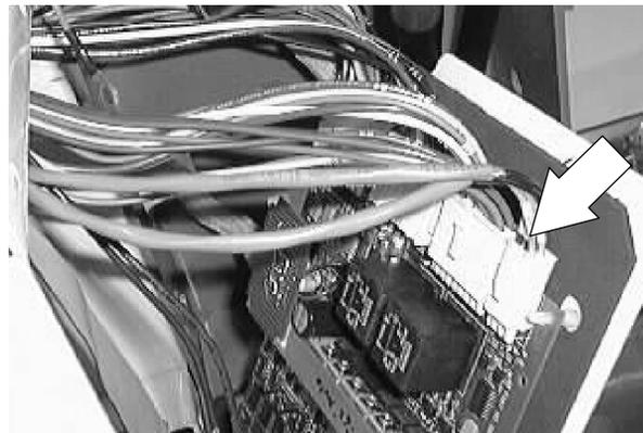
6. Unplug the ribbon cable from the circuit board.
