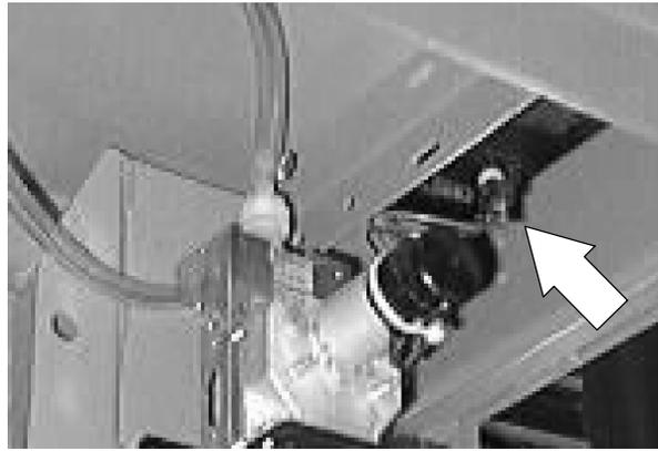
5. Mark and disconnect the two hoses leading to the top of the detergent pump.
