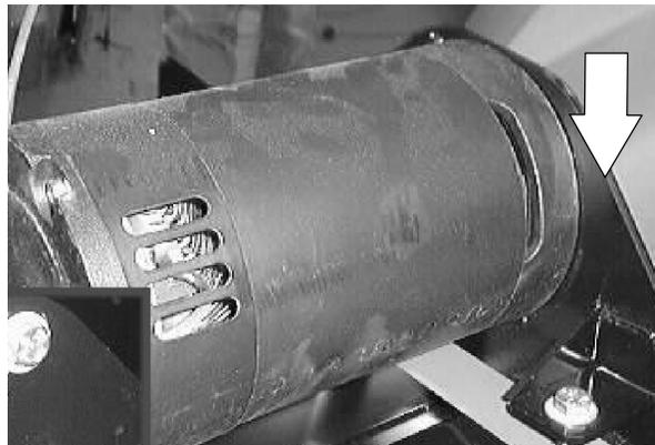
7. Remove the cogged drive belt from the grooved pulley on the brush motor.
