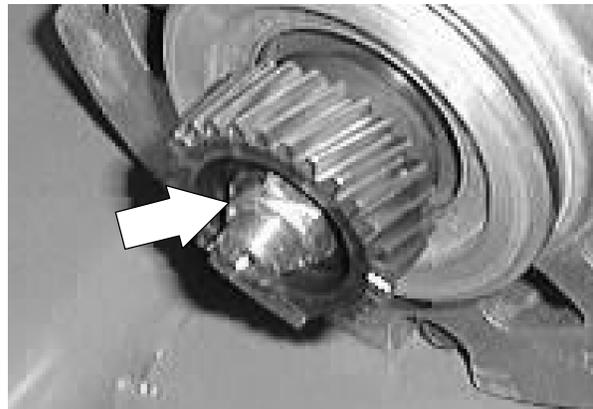
11. Place the gear and key on the new motor shaft. Tighten to 14 - 18 Nm (10 - 13 ft lb).
