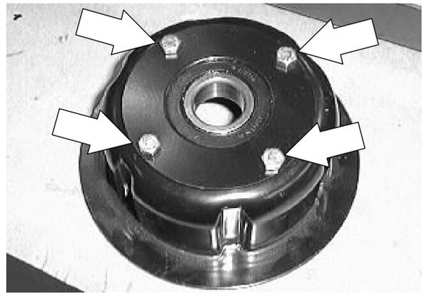
6. Remove the retainer plate to expose the idler bearing.
