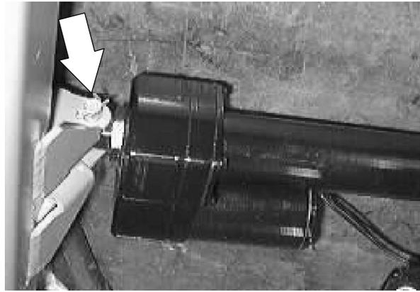
5. Go in to the center of the scrub head. Disconnect the scrub head lift actuator from the main harness.
