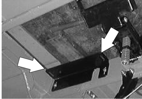
8. Remove the two hex screws holding battery cover mount plate to the inside of the solution tank.
