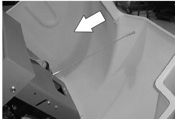
11. Plug the battery connector into the machine. Close the rear cover.
