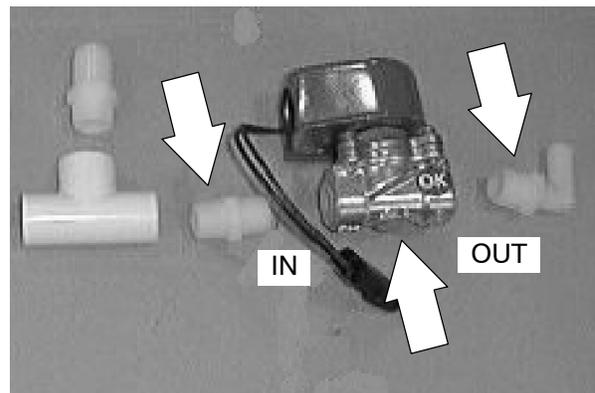
12. Reinstall the autofill valve assembly and retainer bracket onto the pump mount bracket. Reinstall the three hex screws and tighten to 11 - 14 Nm (7 - 10 ft lb).
