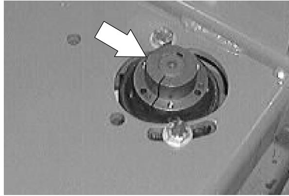
9. Mark, disconnect, and plug the two hydraulic hoses leading to the steering motor.
