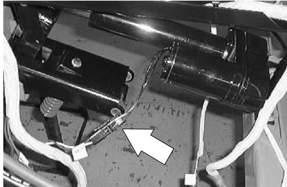
11. Operate the machine. Check the scrub head lift actuator for proper operation.
