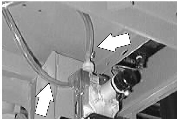
6. Remove the two hex screws holding the detergent pump to the mount bracket. Remove the pump from the machine.
