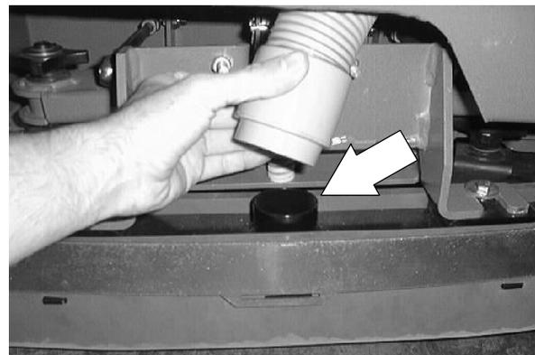
4. Turn the hex screw in the center of the squeegee mount bracket to adjust the tips up or down.
