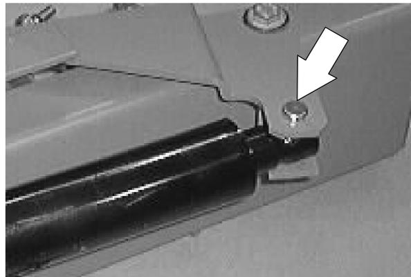
8. Position the new rear squeegee lift actuator onto the front of the squeegee mount frame.
