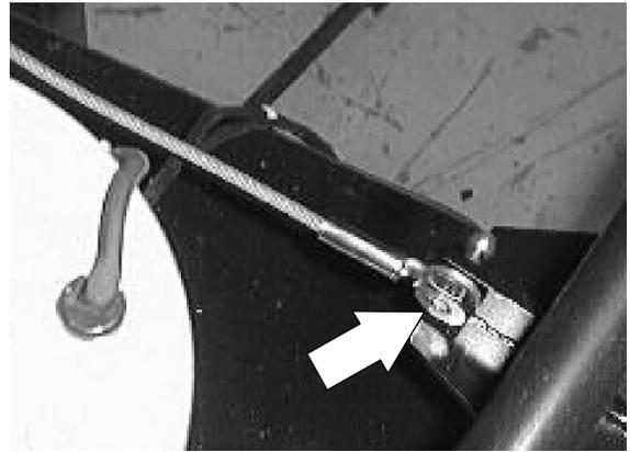
10. Remove the cotter pins and castle nuts from the end of the scrub head drag links where they attach to the machine frame.
