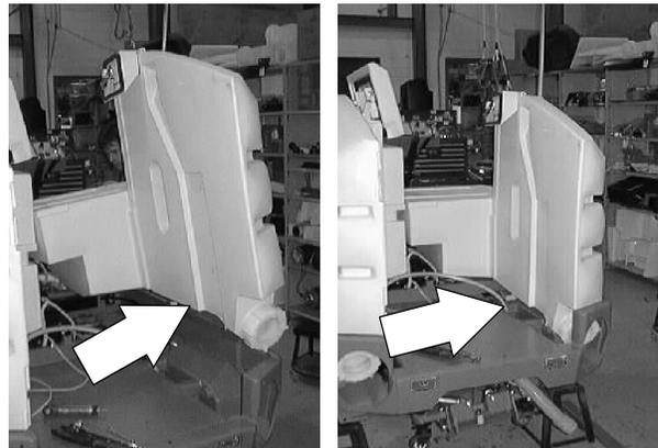
2. Loosely install the two hex screws holding the solution tank to the vertical mount channel at the right side of the battery.
