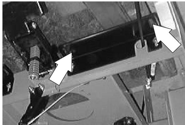
9. Remove the bracket holding the rear squeegee vacuum hose to the side of the recovery tank. Remove the vacuum hose from the recovery tank.
