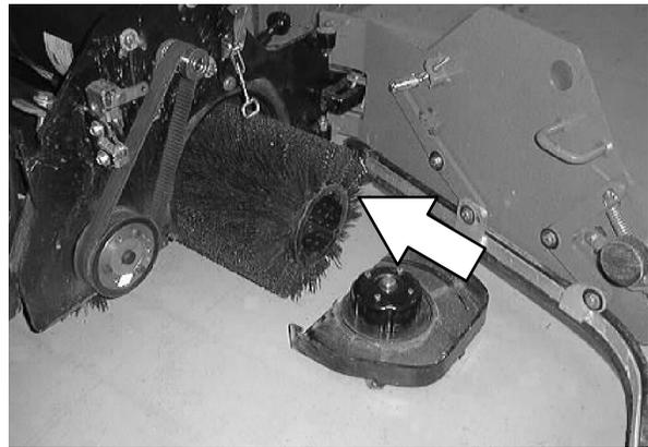
19. Operate the machine. Check the scrub brush motor for proper operation.
