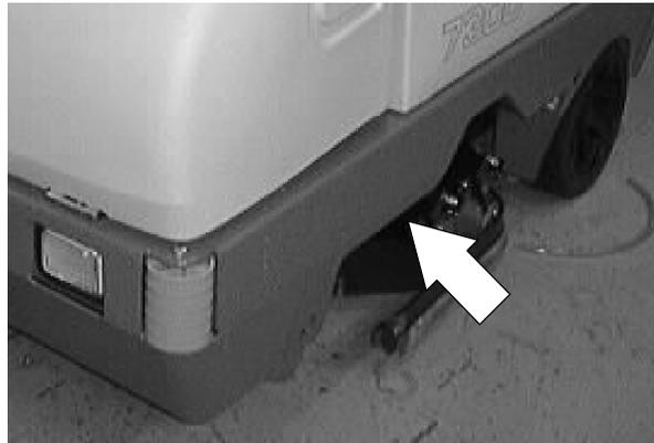
3. Locate the scrub head side shift actuator above the front of the scrub head.
