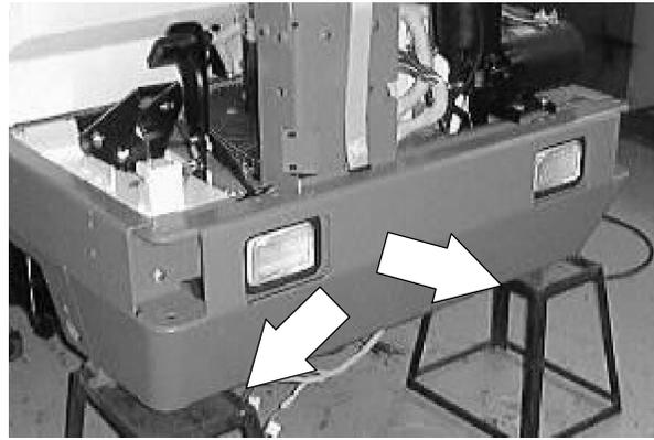
15. Push or pull the scrub head out the right side (operators compartment side) of the machine. The scrub head can now be removed from the machine.
