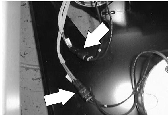
3. Go under the scrub head and remove the hex screw holding the scrub brush drive plug to the brush motor.
