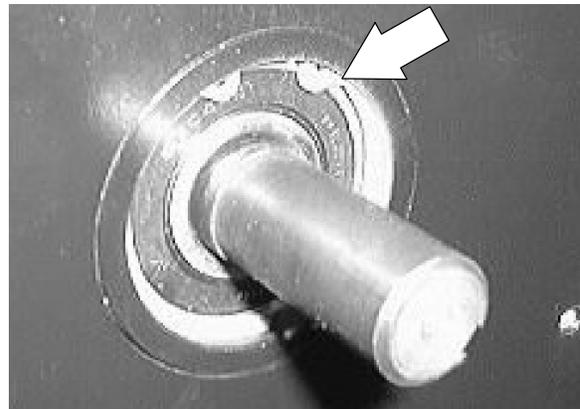
7. Remove the screw and washer holding the scrub brush drive plug to the shaft.
