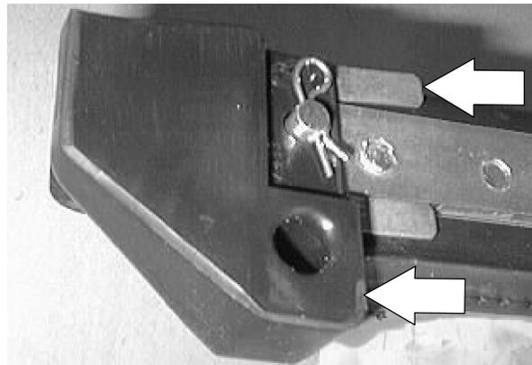
6. Reinstall the clevis pin and hair pin.
