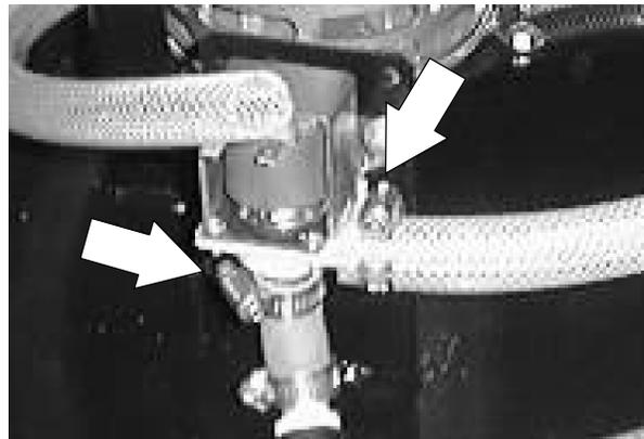
7. Remove the two screws holding the solenoid valve to the mount bracket. Remove the solenoid valve from the machine.
