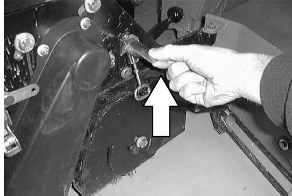
2. Remove the cogged drive belt from the scrub brush drive sheave. See TO REPLACE CYLINDRICAL SCRUB HEAD BRUSH MOTOR instructions in the ELECTRICAL section.
