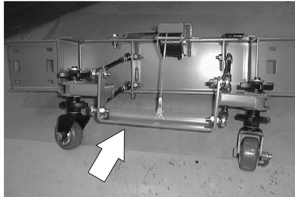
3. Reinstall the hardware. Tighten to 37 - 48 Nm (26 - 34 ft lb).
