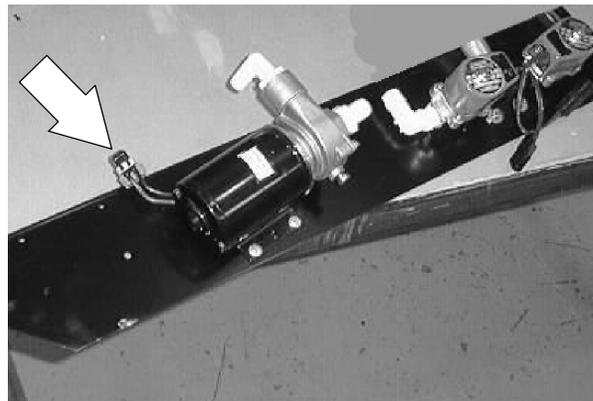
4. Loosen the wormdrive clamp holding the recovery tank hose to the ES™ pump center fitting. Pull the hose off the fitting.
