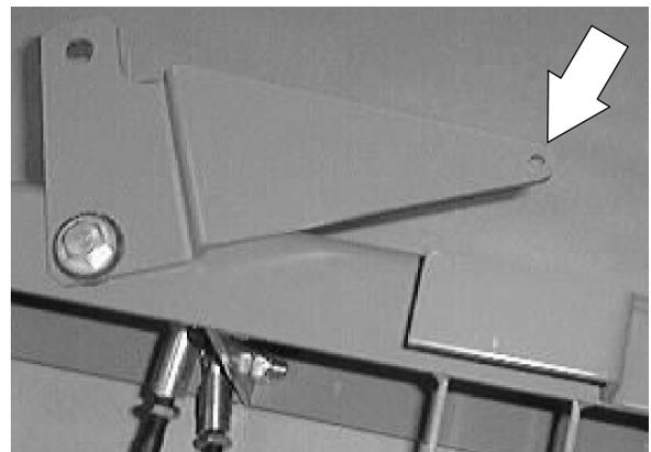
8. Reattach the squeegee lift cable to the actuator squeegee lift bracket using the clevis pin and cotter pin.
