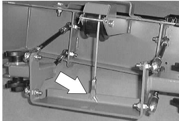
3. Remove the cotter pin and clevis pin from the squeegee lift cable where it attaches to the actuator lift pivot bracket.
