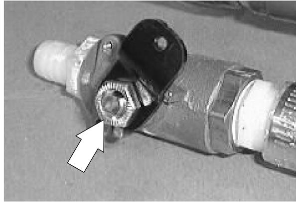
8. Install the new valve assembly onto the mount bracket. Reinstall the hardware and tighten hand tight.
