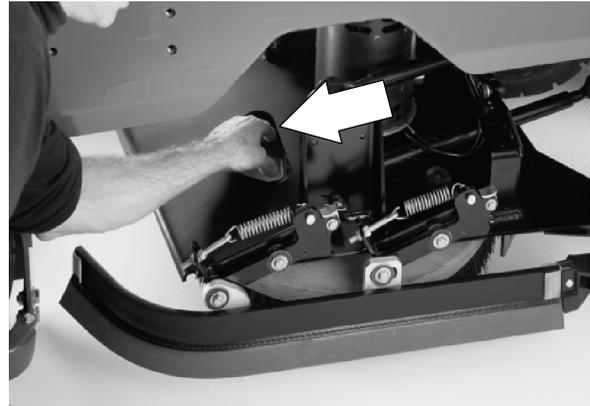
The scrub brushes should be checked daily for tangled wire or string wear damage. The scrub brushes should be replaced if large portions of the brush bristles are missing or if the remaining brush bristle measure 0.38 in (10 mm) or less in length.
