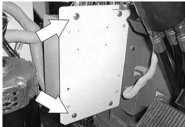
4. Pull the small control panel cover back to access the circuit board (s).
