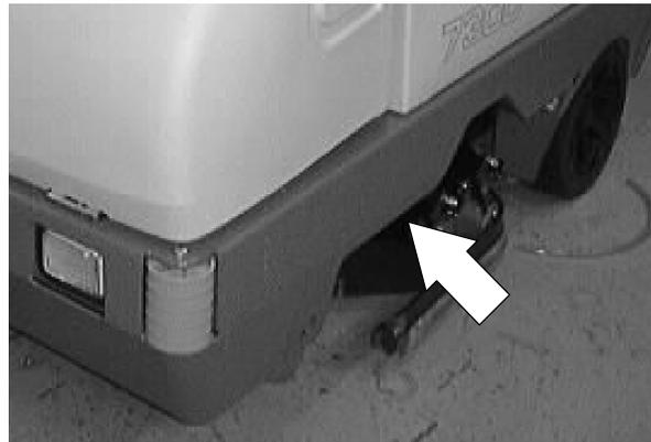
3. Locate the detergent pump on the left hand frame leg.
