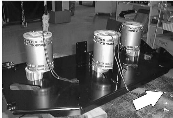
3. Position the two scrub head drag links into the frame mount holes.
