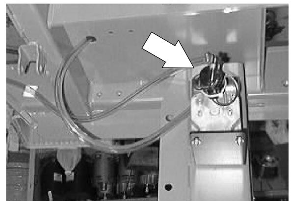
8. Reconnect the two hoses leading to the top of the detergent pump.
