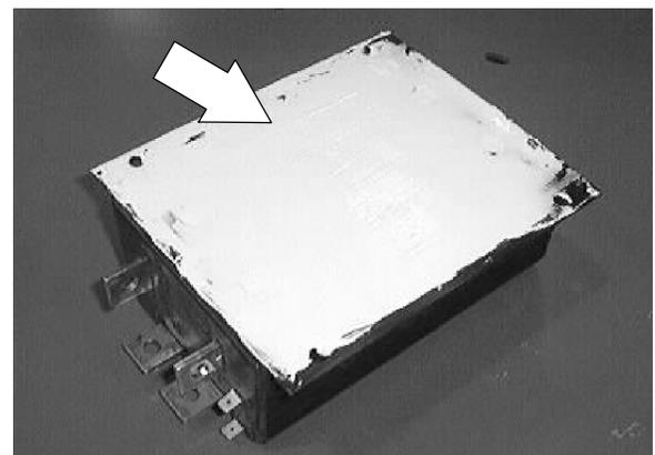
8. Install the new controller onto the control panel. Reinstall the four hex screws. Tighten to 7.6 - 9.9 Nm (5 - 6 ft lb).
