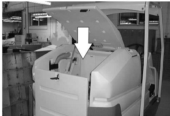
3. Go to the operators compartment and remove the cotter pin and clevis pin from the actuator where it attaches to the scrub head lift pivot bracket.
