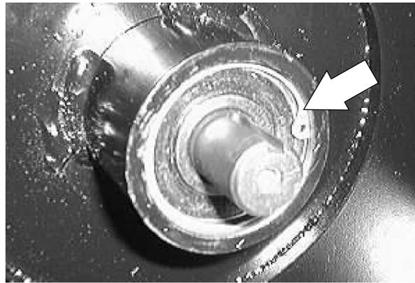
10. Use a rubber hammer to tap the shaft and bearing assembly out of the bearing housing (*tap the assembly into the center of the scrub head*). **Note the orientation of the shaft in the housing.**
