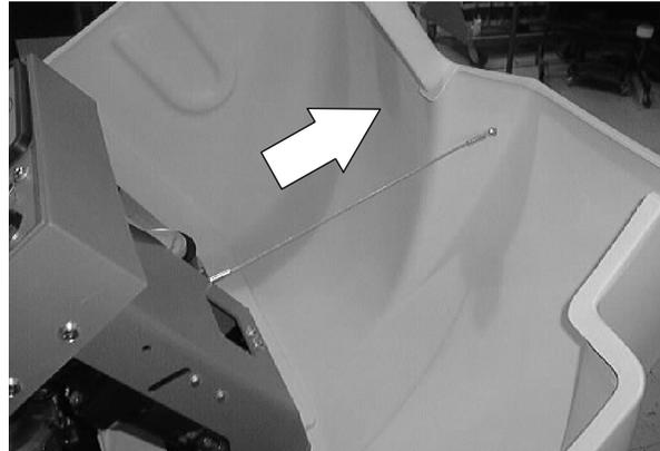
2. Locate the manual solution valve push/pull cable on the left side of the steering column.
