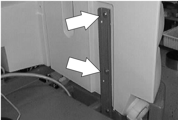
10. The solution tank can now be carefully be lifted out of the machine frame.
