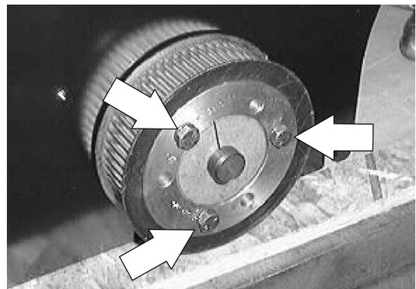
4. Screw the three hex screws into the open holes on the cogged sheave and tighten. This will push the cogged sheave off the shaft hub
