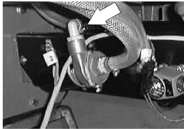
10. Reinstall the recovery tank hose onto the lower fitting on the ES™ pump. Tighten the wormdrive clamp.
