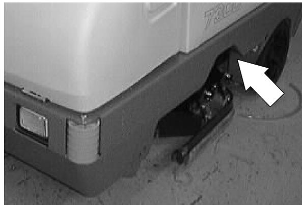
4. Locate the autofill valves on the mount bracket between the rear wheels.
