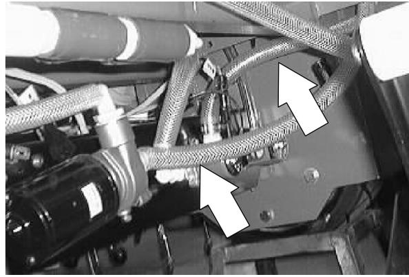
8. Go under the recovery tank in the area under the scrubbing vacuum fans. Remove the two hex screws holding the front of recovery tank to the frame bracket.
