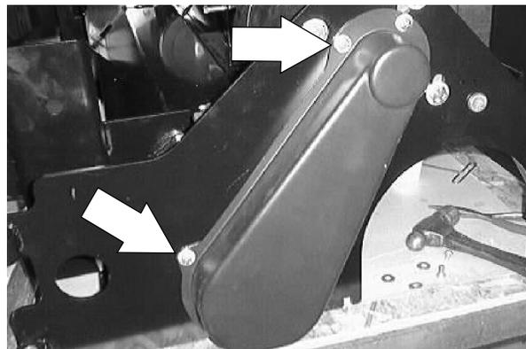
4. Loosen the four hex screws holding the scrub brush motor to the scrub head.
