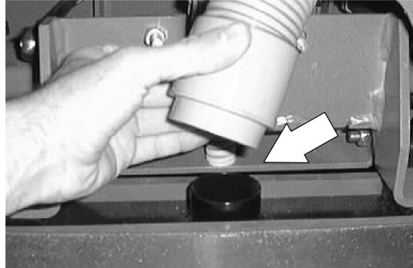
2. Loosen the hardware holding the squeegee frame to the lift assembly. Pull the squeegee frame and blade assembly off the machine.
