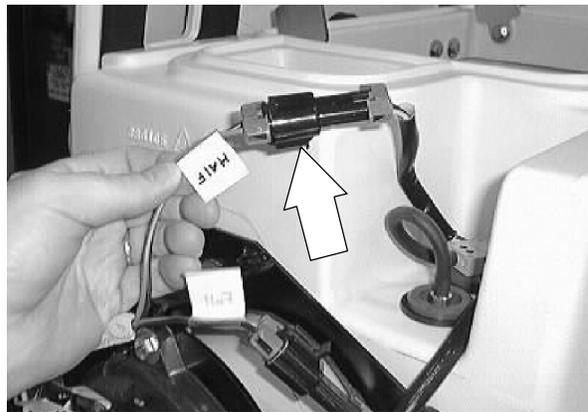
5. Disconnect the scrubbing vacuum fans and vacuum switch from the main harness.
