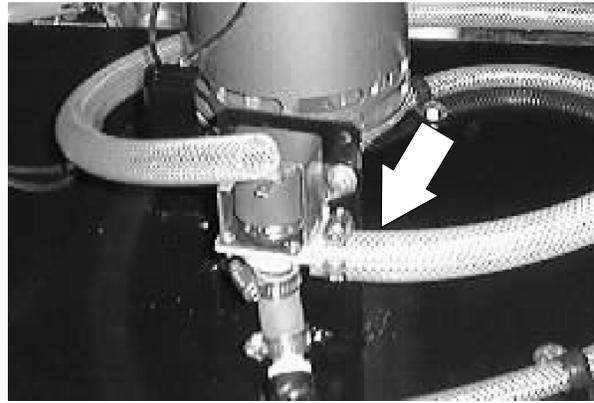
8. Disconnect the end of the side shift gas spring where it attaches to the scrub head.
