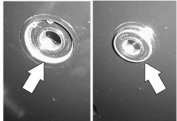
12. Install the new bearings and shaft assembly into the bearing housing (*tap the assembly into the housing from the center of the scrub head to the outside of the scrub head*). **The longer shaft end goes to the outside of flange.**
