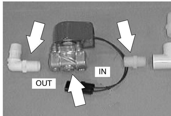
11. If replacing right hand autofill valve--note orientation of valve and fittings.
