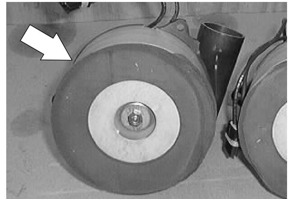
7. Position the new vacuum fan onto the fan mount bracket.
