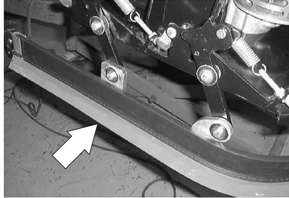
2. Remove the plastic tip and metal retainer.
