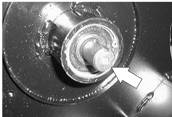
13. Reinstall both bearing snap rings.
