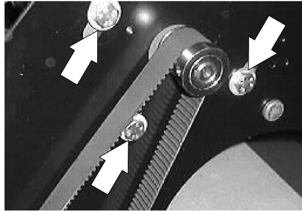
5. Loosen the hex screws holding the brush motor support strap to the mount bracket.
