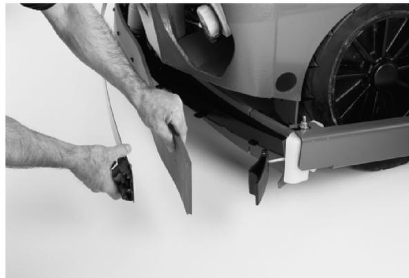
5. Install the new or rotated blade onto the squeegee frame.
