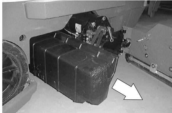
3. Go under the machine in the area of the center of the scrub head. Remove the hex screw holding the **UPPER** head lift roller to the mount bracket. Remove the roller from the scrub head frame.
