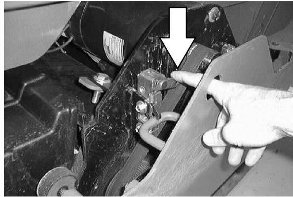
7. While holding the smaller hex, loosen the larger mounting screw on the outside of the idler door.
