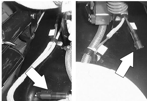
6. Reconnect the water flow solenoid to the main harness.
