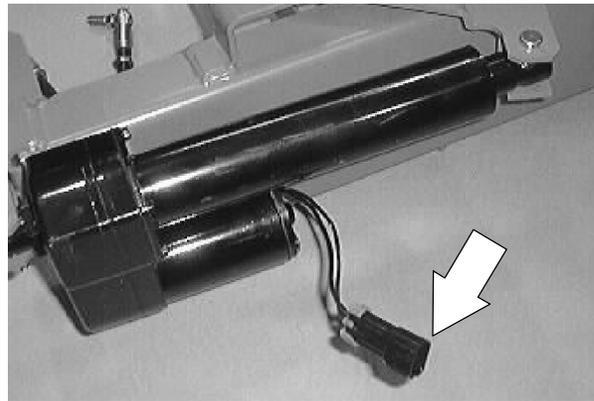
6. Remove the cotter pin and clevis pin from the motor end of the actuator where it attaches to the squeegee mount frame.
