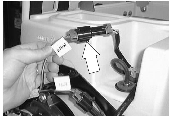
11. Plug the battery connector into the main connector.
