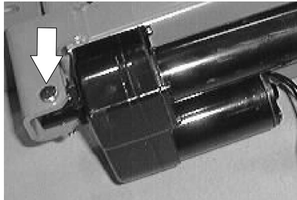
7. Remove the cotter pin and clevis pin from the rod end of the actuator where it attaches to the squeegee lift cable pivot bracket. Remove the actuator from the machine.
