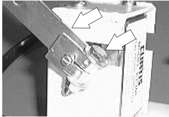
9. Position the new Curtis accelerator unit on the mount bracket. Reinstall the two pan screws and tighten to 7.6 - 9.9 Nm (5 - 6 ft lb). *Make sure the wire harness is placed through the grommet and the grommet is installed in the hole of the floor plate.*
