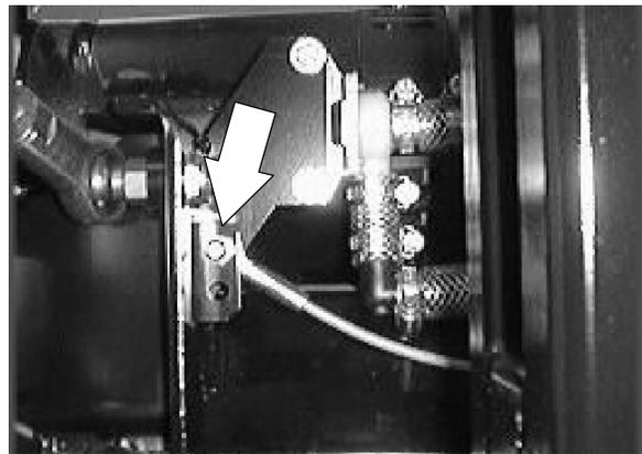
11. Remove the cotter pins and castle nuts from the end of the **LOWER** scrub head drag links where they attach to the machine frame.
