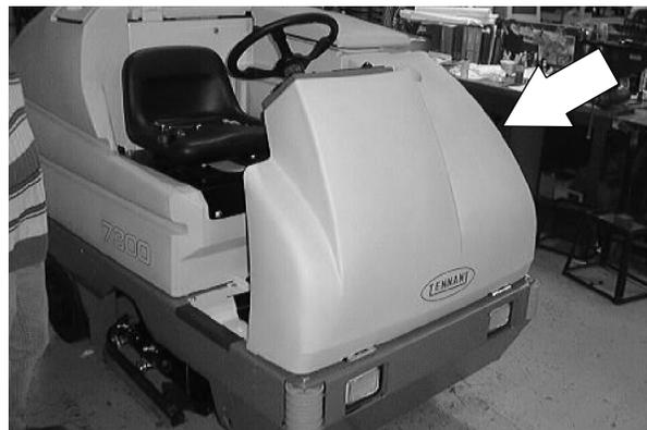
19. Lower the machine to the ground and check the new traction motor for proper operation.
