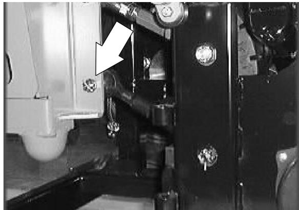
12. Remove the larger nyloc nut from the **UPPER** scrub head drag links where they attach to the machine frame.
