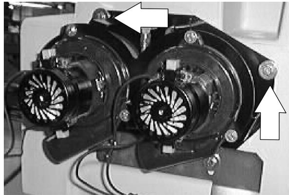
6. Remove the vacuum fan assembly from the machine.
