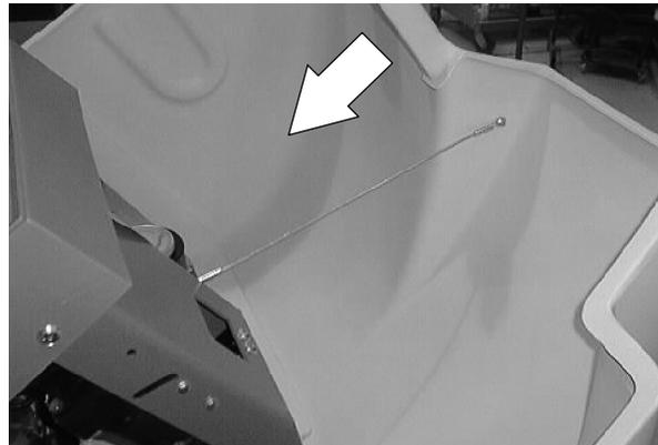
18. Plug the battery connector into the machine. Close the rear cover.
