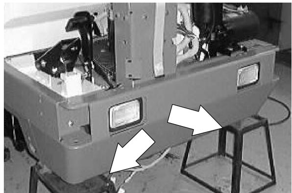
13. Push or pull the scrub head out the right side (operator's compartment side) of the machine. The scrub head can now be removed from the machine.
