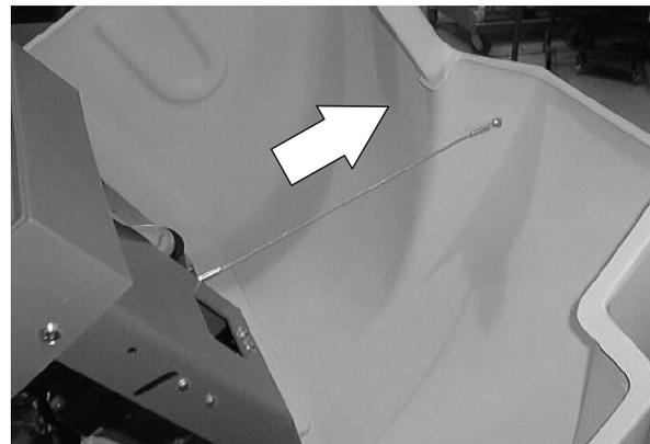
3. Remove the detergent tank and main control panel cover from the machine.
