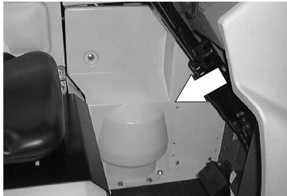
20. Plug in the battery connector. Close the battery cover.
