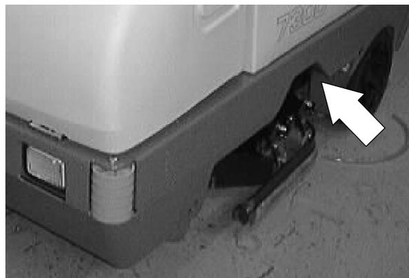
4. Locate the solution solenoid valve in the center, front area of the scrub head.
