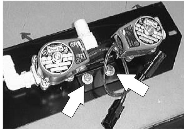
13. Reconnect the three hoses to the autofill valve assembly.
