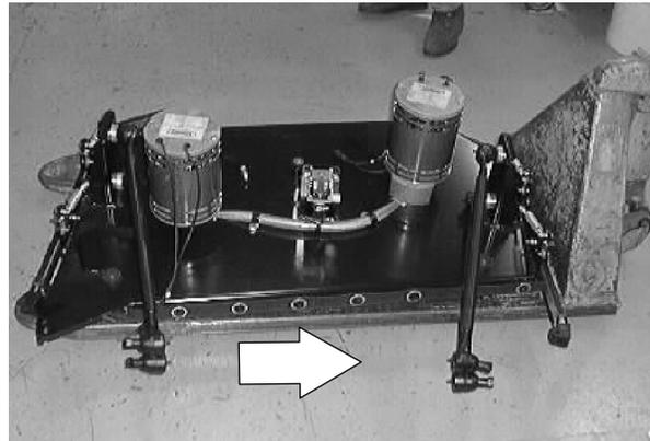
3. Position the four scrub head drag links into the frame mount holes.
