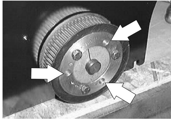
5. Loosen the set screw holding the shaft hub to the square key and shaft.
