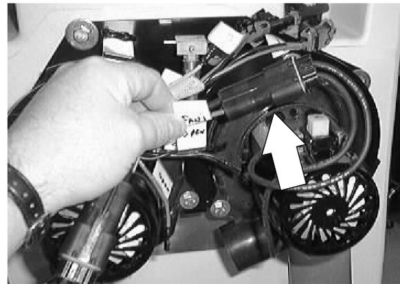
10. Plug the battery into the connector.
