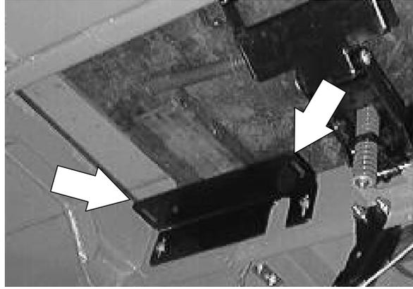
5. Reinstall the seat assembly. Reinstall the six hex screws holding the operator seat mount plate to the solution tank. Tighten screws to 18 - 24 Nm (15 - 20 ft lb).
