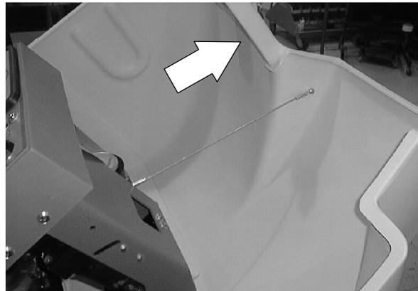
3. Disconnect the two wires leading to the electro/hydraulic motor.
