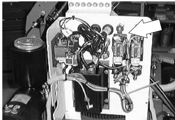
5. Loosen the two hex screws holding the propelling fuse to the cable standoffs.
