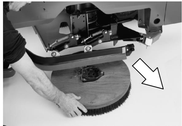
6. Position the new scrub brush under the scrub head. Line up the motor drive plug with the brush drive insert.
