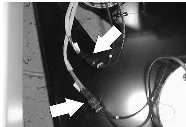
6. Disconnect the main harness from the water flow solenoid.
