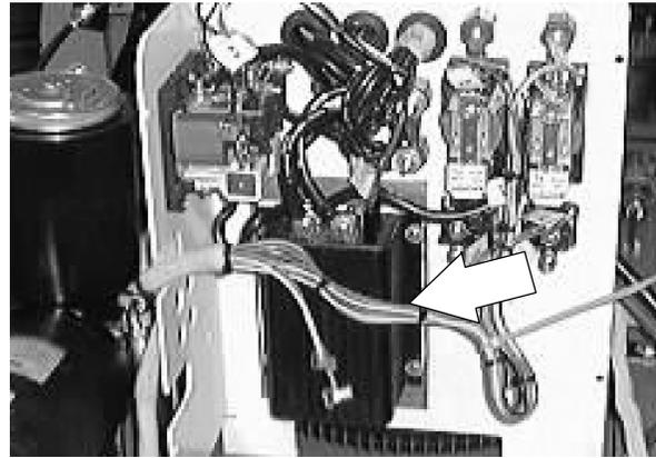
5. Mark and disconnect the electrical cables and smaller wires leading to the top of the controller.
