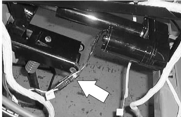
*NOTE: Use the "Manual Mode" to extend/retract the new actuator for installation.*
