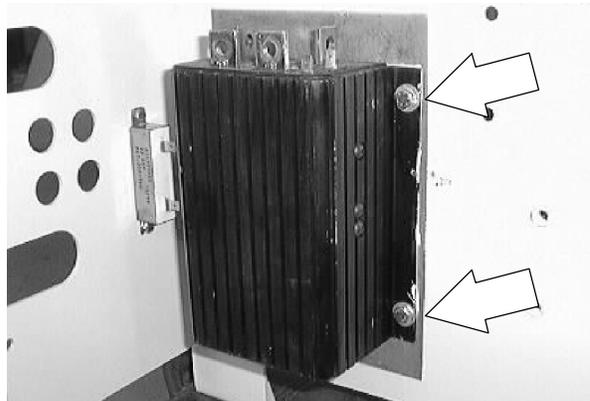
7. Cover the back side of the new controller with electrical thermal grease.
