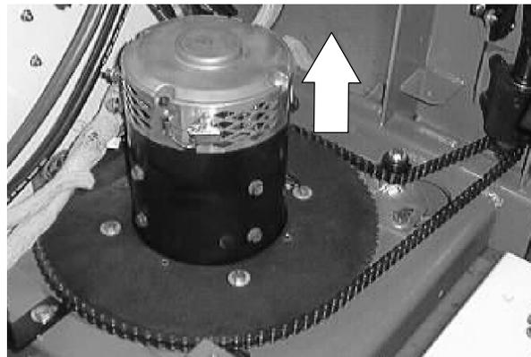
10. Remove the 0.50 in x 20 thin nyloc holding the drive gear to the motor shaft.
