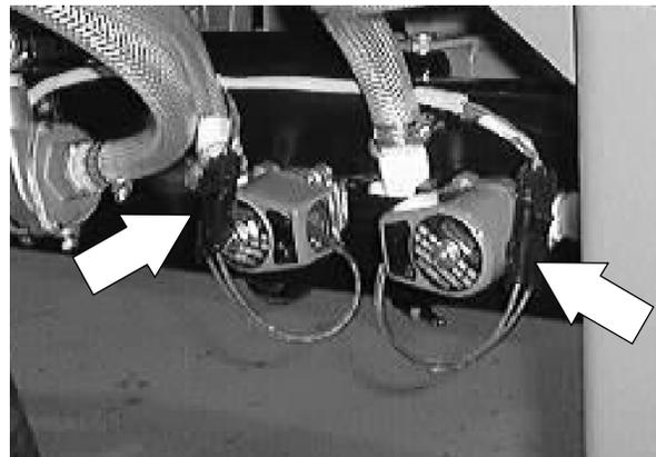
15. Operate the machine and check the new autofill valve for proper operation.
