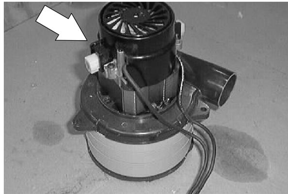
6. Check the gasket on the back of the vacuum fan for rips or tears before installing on the mount bracket.
