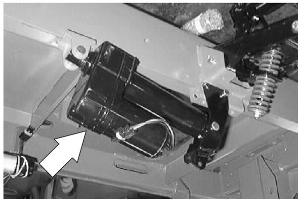
4. Disconnect the side shift actuator from the main harness.
