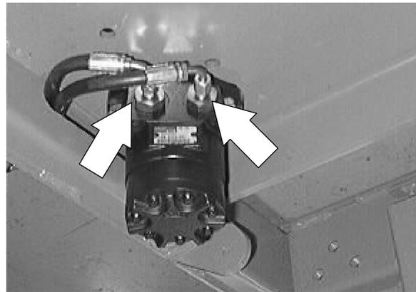
10. Remove steering motor hardware. Remove the motor from the machine.
