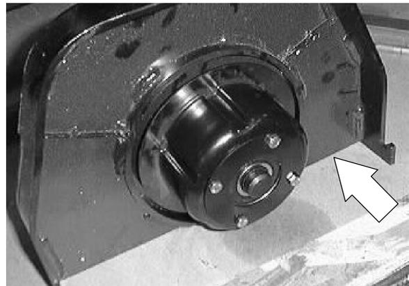
3. Remove the hex screw holding the brush idler plug and cam assembly to the mount plate.
