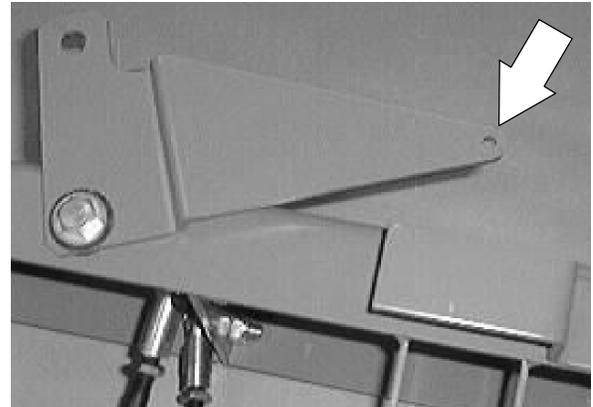
4. Remove the cotter pin from the long clevis pin in front of the squeegee lift cable roller. Remove the clevis and the lift cable from the machine.
