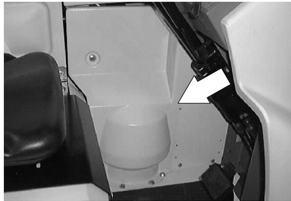
6. Mark and disconnect the four electrical cables leading to the traction motor.
