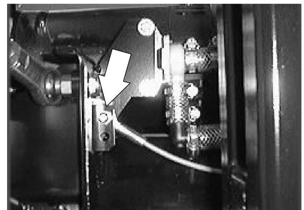
13. Reconnect the end of the side shift gas spring where it attaches to the scrub head. Reconnect the kick-in guard to the front, right corner of the scrub head.
