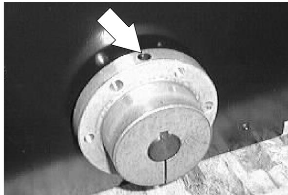
16. Position the cogged sheave onto the shaft hub. Reinstall the three hex screws. Tighten to 8 - 10 Nm (5 - 7 ft lb).
