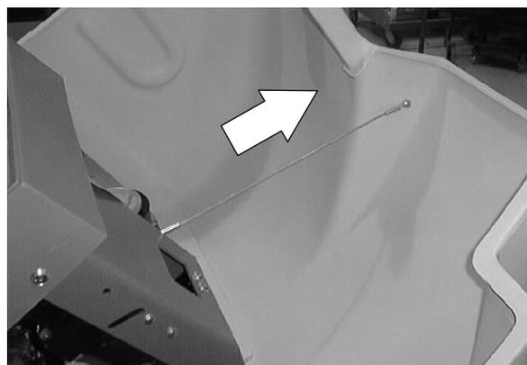
3. Remove the detergent tank and main control panel cover from the machine.
