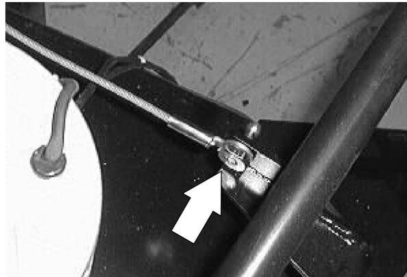
10. Remove the cotter pins and castle nuts from the end of the scrub head drag links where they attach to the machine frame.
