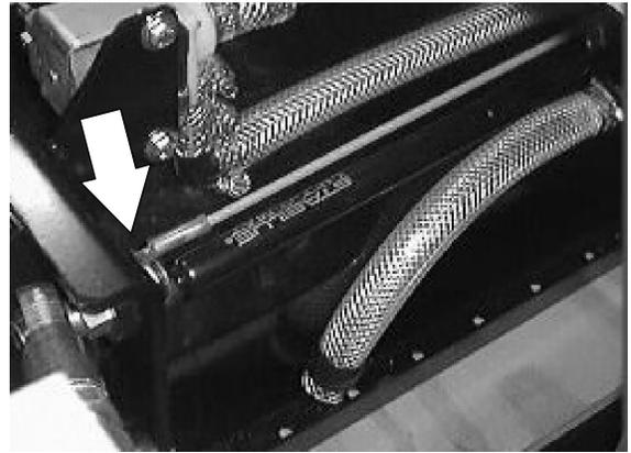
10. Disconnect the end of the side shift cable where it attaches to the scrub head.
