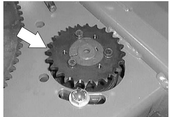
15. Use a straight edge to align the small sprocket with the large sprocket. Tighten the three hex screws to 11 - 14 Nm (7 - 10 ft lb). *Use loctite blue 242 on the threads.*
