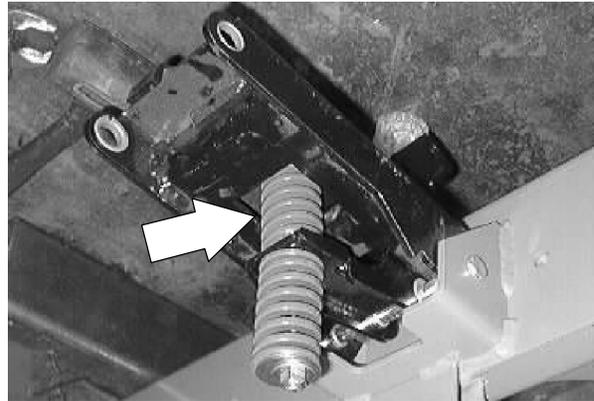
**IF ACTUATOR FAILED WITH SCRUB HEAD IN THE LOWERED POSITION:** (*Bottom die spring compressed and actuator is retracted*).
