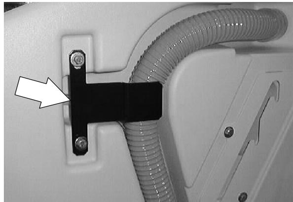
10. Remove the two hex screws holding battery cover mount plate to the inside of the recovery tank.
