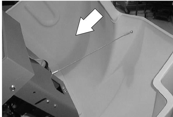
10. Plug the battery connector into the machine.
