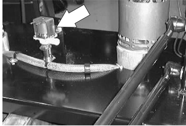
5. Disconnect the solenoid valve from the main harness.
