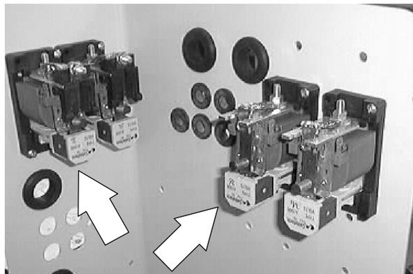
8. Reconnect the electrical cables and smaller wires leading to the top of the 36V relay.
