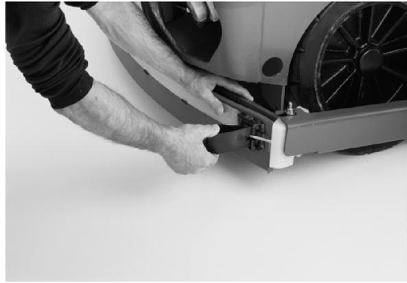
4. Pull the rubber squeegee blade off the frame. Rotate the blade to one of the four edges or discard blade.
