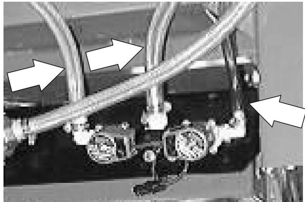
14. Reconnect the valve solenoids to the main harness.
