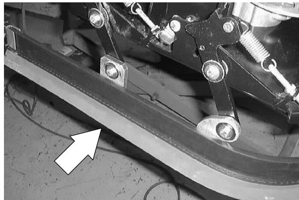
5. Reinstall the metal retainer and plastic tip.
