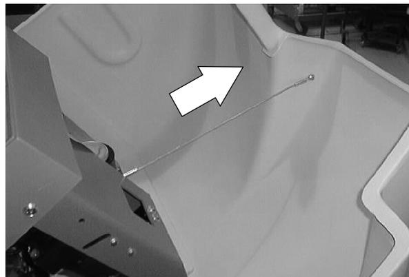
3. Remove the detergent tank and control panel cover from the machine.
