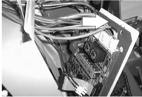
5. Unplug the wire connectors on top of the circuit board.
