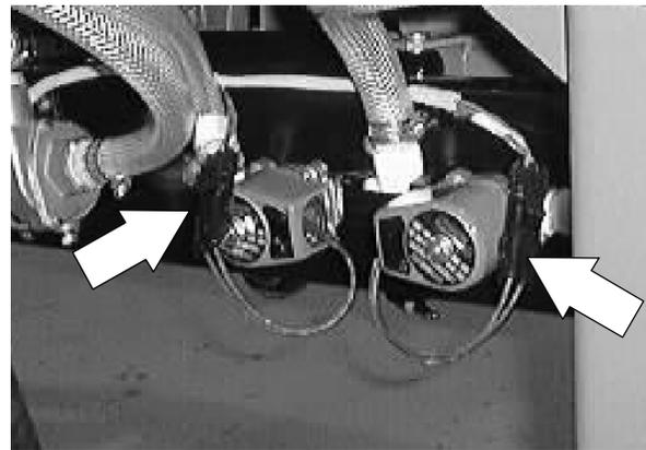
6. Mark and disconnect the three hoses leading to the autofill valve assembly.
