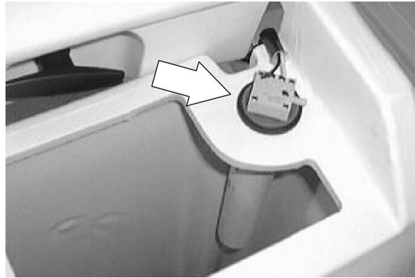
9. Plug the battery connector into the main connector.
