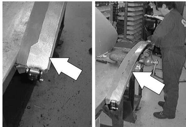
7. Flip the squeegee band lock into place and snap down to lock.
