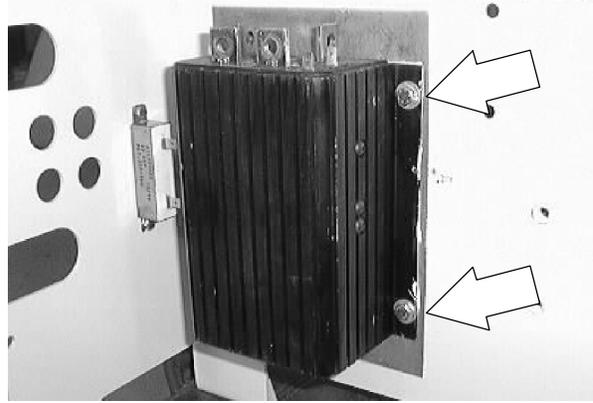
9. Reconnect the electrical cables and smaller wires leading to the top of the controller.
