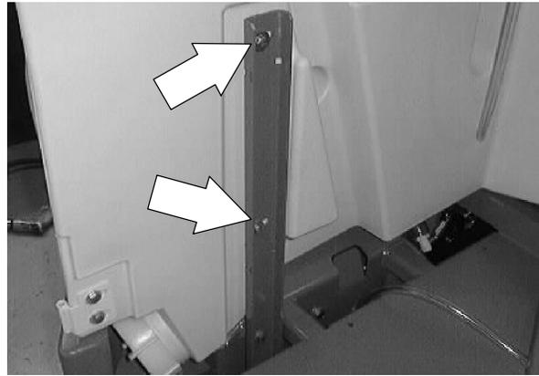
12. Remove the clamp holding the battery cables to the back of the recovery tank.
