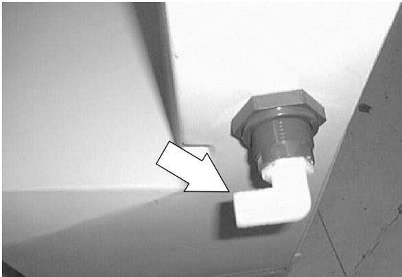
7. Reconnect the ES™ water line to the top of the solution tank. (*ES™ option only*)
