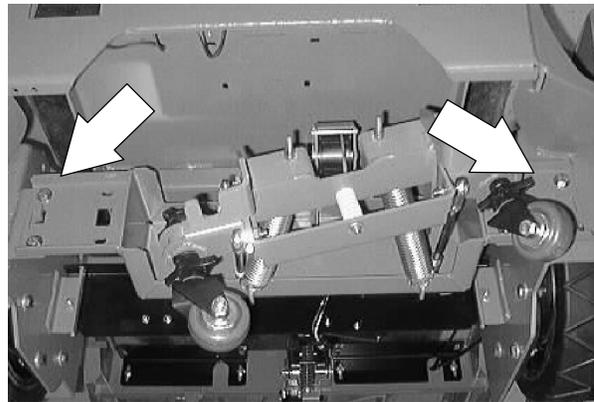
4. Reinstall the squeegee blade assembly frame onto the lift bracket. Position the vacuum hose into the hole in the squeegee frame.
