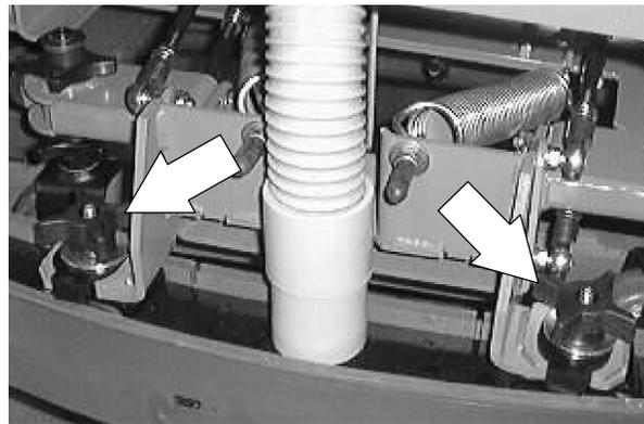
3. Remove the four hex screws holding the rear squeegee assembly to the machine frame.
