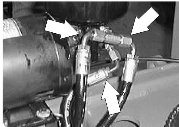
5. Remove the four M8 hex screws holding the electro/hydraulic unit to the machine frame.
