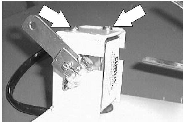
7. Loosen the hex screw and nut holding the lever and rod to the Curtis accelerator unit. Remove the lever and rod assembly from the unit.
