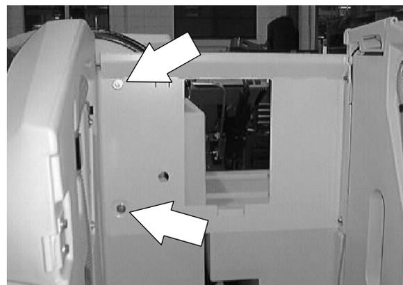
11. Remove the two hex screws holding the recovery tank to the vertical mount channel at the left side of the battery.
