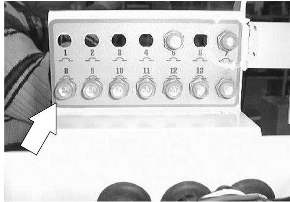
5. Mark and disconnect the wire leading to the circuit breaker that needs to be changed.
