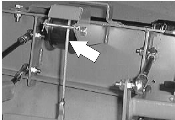
6. Reinstall the clevis pin and cotter pin in front of the lift roller.
