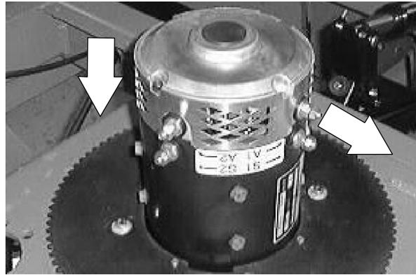
13. Reinstall the three M8 socket head cap screws holding the traction motor to the drive gear box. Tighten to 26 - 34 Nm (20 - 26 ft lb).
