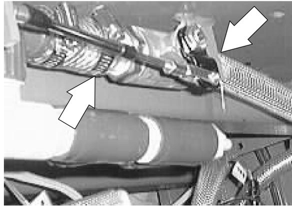
4. Remove the cotter pin and clevis pin holding the push/pull cable clevis to the manual valve lever.
