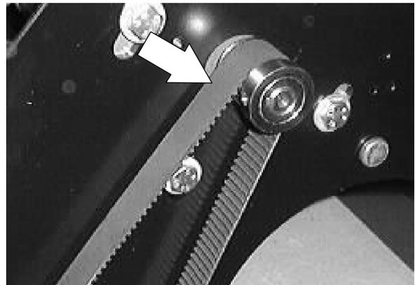
13. Use the brush motor support strap to move the brush motor up to tighten the cogged belt. Tighten the strap hex screw to 18 - 24 Nm (15 - 20 ft lb).
