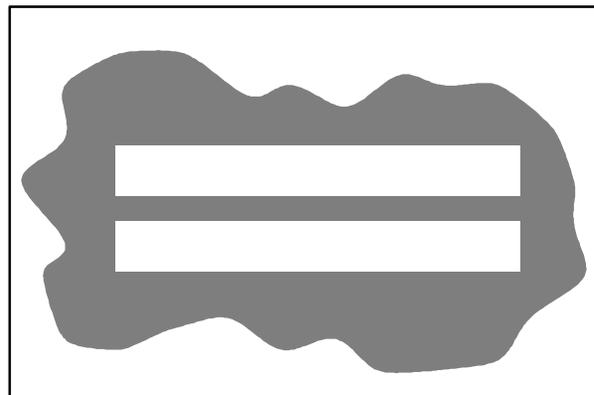
If one, or both of the brush patterns are tapered, the brushes need adjustment to straighten the brush pattern.
