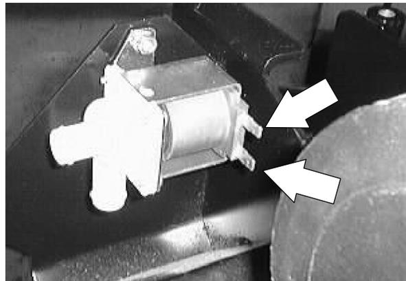
8. Disconnect the solution line from the water flow solenoid.
