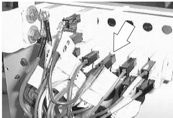
6. Remove the rubber boot from the outside of the circuit breaker. Remove the circuit breaker from the machine.
