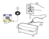
Filling Buckets and Equipment: Turn selector knob to the bucket fill position for MultiMicro 200. Unhook bucket/equipment fill hose from dispenser and insert into container to be filled. Push the dispenser button to fill the container. The dispenser button can be locked into position for filling large containers. Tap the dispenser button to unlock. Refer to the MultiMicro 200 bottle label for instructions for use. Do not dilute with tap water.
