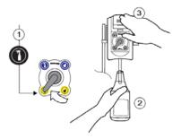
Filling bottles: Turn selector knob to the bottle-fill position for MultiMicro 200. Insert bottle fill nozzle into the spray bottle. Push the dispenser button to fill the bottle. Only use clean bottles properly labeled with labels provided with this machine. Do not use non-labeled or mis-labeled bottles. Refer to the MultiMicro 200 bottle labels for instructions for use. Do not dilute.
