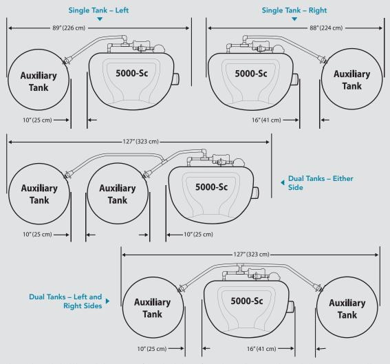
5000-Sc unit and any auxiliary tanks should be installed on an even surface so that the bases of a complete installation are at the same level. A 16" gap is required between an auxiliary tank and the right (inflow filter) side of the tank to allow for access to the inflow filter.
