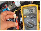
Point the multimeter between pin 1 and 6, the reading is about 3.6 – 3.8V
