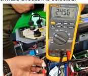
Connect the 6- pins connector with the inverter board, when forward is selected the reading between GND and pin 2 is 0V and the reading between GND and pin 4 and 5 is 24V.
