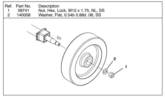
Maximum torque 24 Nm/18 ft-lbs. Do not over tighten nut. Higher torques will deform the center of the wheel, compromising the conical fit to the transaxle.
