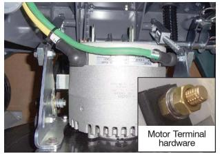
Machines manufactured **AFTER** s/n 10683082, the motor cables are routed as shown below. This reduces the tension at the cable connection points as the head moves up and down. The outside terminal nuts are also Flexlock nuts.
