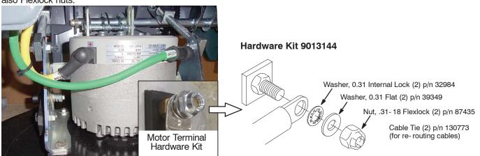
Note: When installing a new motor, remove the terminal hardware that comes installed on motor except for the inside brass nut. Use the hardware kit supplied with new motor as a replacement. Torque both inside and outside nuts to 100 in-lbs (11.3 N-m). Use the cable ties supplied with kit to secure cables as shown above.
