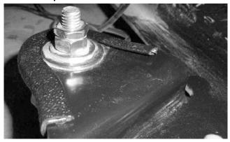
Remove existing protective edging and install longer piece as shown (p/n 1020168).
