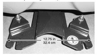
Install upgraded bracket (p/n 1018725). The width of the upgraded bracket measures 12.75" (32.4 cm).
