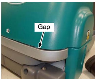
Shroud not properly seated. Gap can be as little as 1/16" (1.5 mm).
