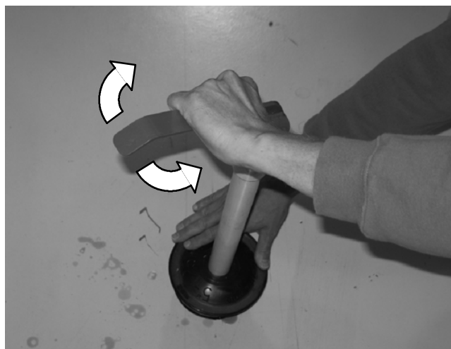
Fig. 4: Turn handle clockwise to expand plug for a tighter fit. Turn handle counterclockwise to contract plug for a looser fit. Be sure to hold onto the plug portion of the drain plug, not the shaft, when turning the handle to tighten or loosen the plug.
