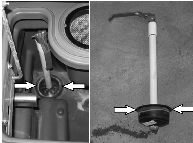
Fig. 3: The plug must be snugly seated in the drain hole and the flange must be flush against the recovery tank floor.
