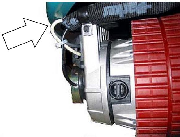
Abrasion point when making a right hand turn. Comes in contact with the scrub head pivot arm.
