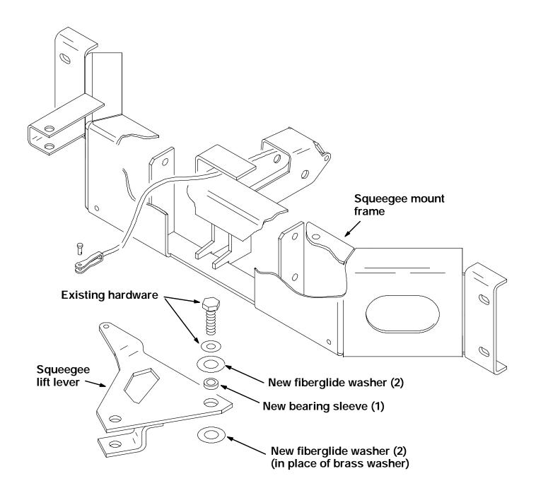
FIG. 1 - Rear Squeegee Lift Lever Assembly
