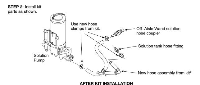
\* **NOTE:** Route the new hose assembly under the ReadySpace vacuum hose and clear solution hose.
