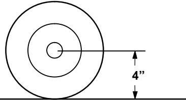
For proper machine operation, inflate air filled tires to a rolling radius of 4".
