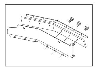
4. Insert the plastic left side **squeegee plate 1008969** in betweeen the sqeegee and mounting plate.
