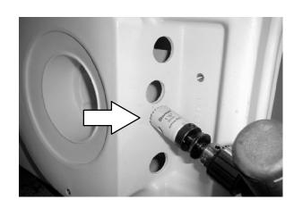
4. Install the bulkhead fitting (9) and elbow (10) to the recovery tank. (Refer to FIG. 2)
