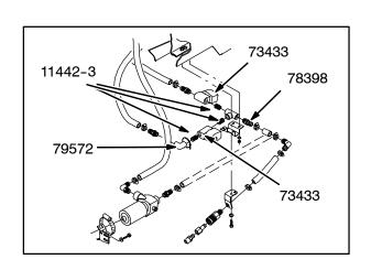
13. Remount the solenoid valve assembly.
