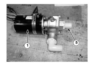
11. Remount the pump (1) assembly to the frame. (Refer to FIG. 1)
