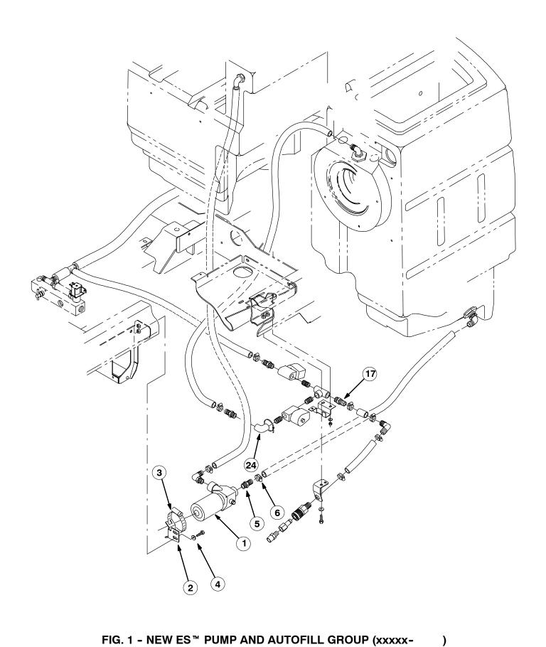
FIG. 1 - NEW ES™ PUMP AND AUTOFILL GROUP (xxxxx-
