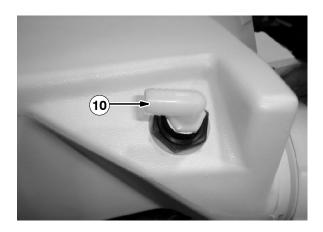
3. Mark and drill a 35mm (1 3/8" dia) hole for the recovery tank autofill.
