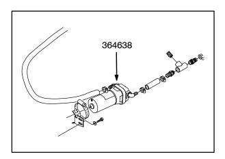
2. Remove all of the hoses, tees, elbows and solenoids in the ES<sup>™</sup> system. Leave the autofill fittings up to the first tee fitting.
