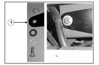
7. Connect the main brush lift cable 383194 to the new lift lever (1) with set aside mounting hardware.
