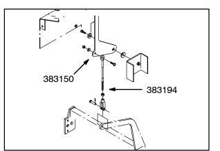
3. Disconnect lift lever 383150 from the machine. Set the mounting hardware aside.
