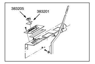
5. Remove and discard the main brush panel 383215 and lift handle seal 383196.
