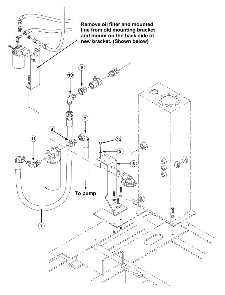
FIG. 2 - NEW HYDRAULIC LINE INSTALLATION
