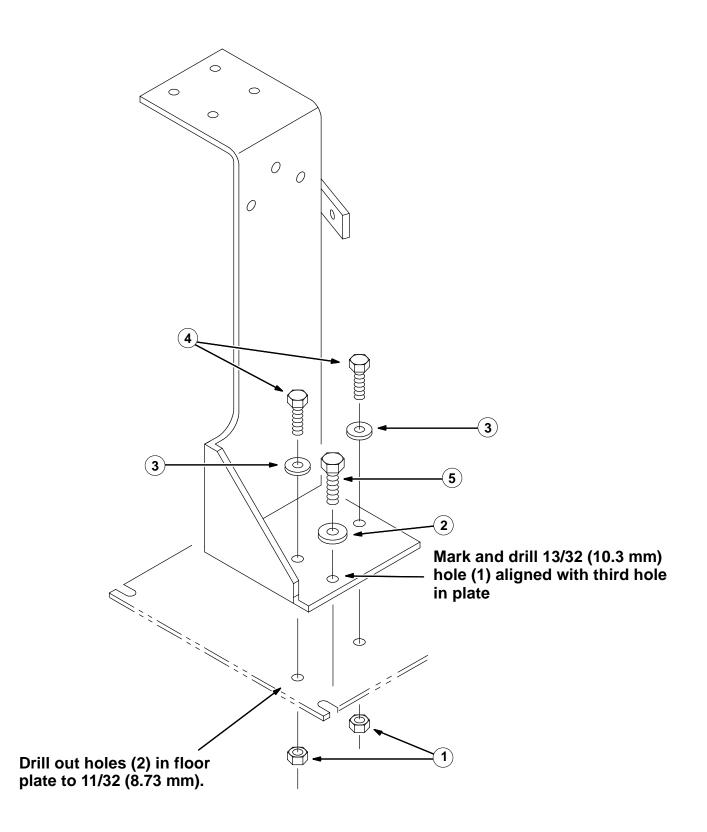
FIG. 1 - NEW MOUNTING BRACKET INSTALLATION
