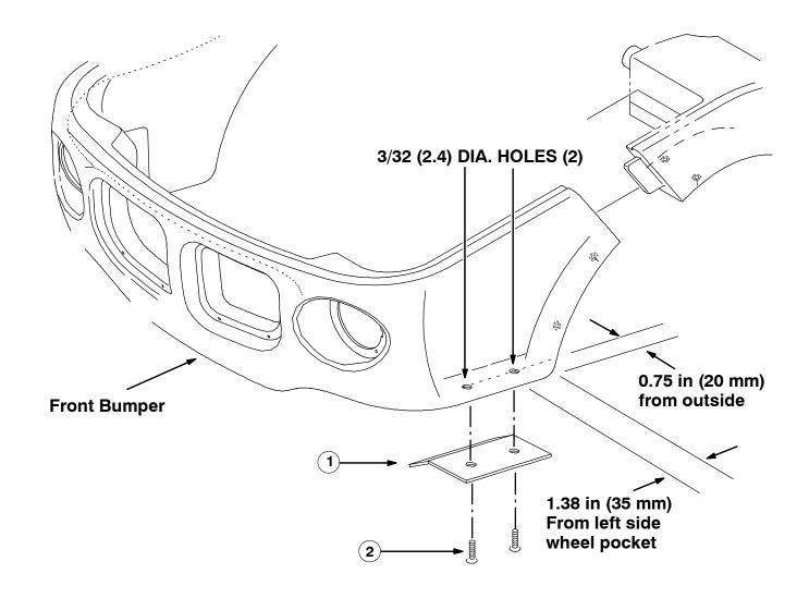
FIG. 1 - DEFLECTOR ANGLE INSTALLATION
