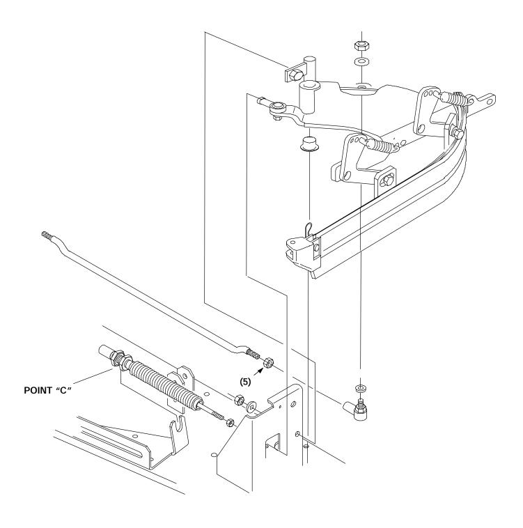
FIG. 1 - Replacement of Side Squeegee Assemblies and Installation of Side Squeegee Stabilizing Rod on <u>Left Hand</u> Side of Machine
