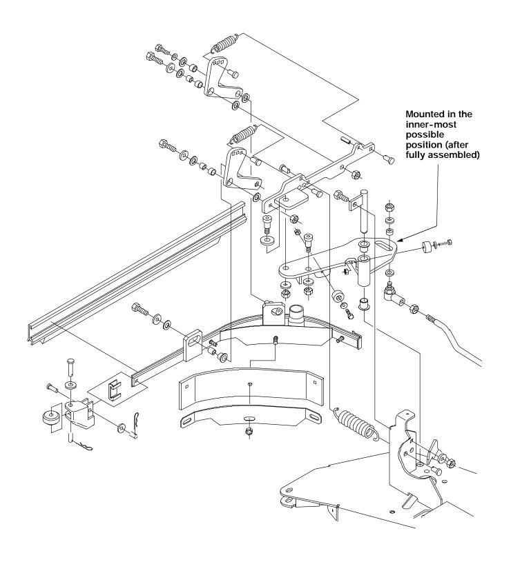
FIG. 2 - Installation of Side Squeegee Stabilizing Rod on <u>Right Hand</u> Side of Machine BILL OF MATERIALS FOR KIT NUMBER 365144
