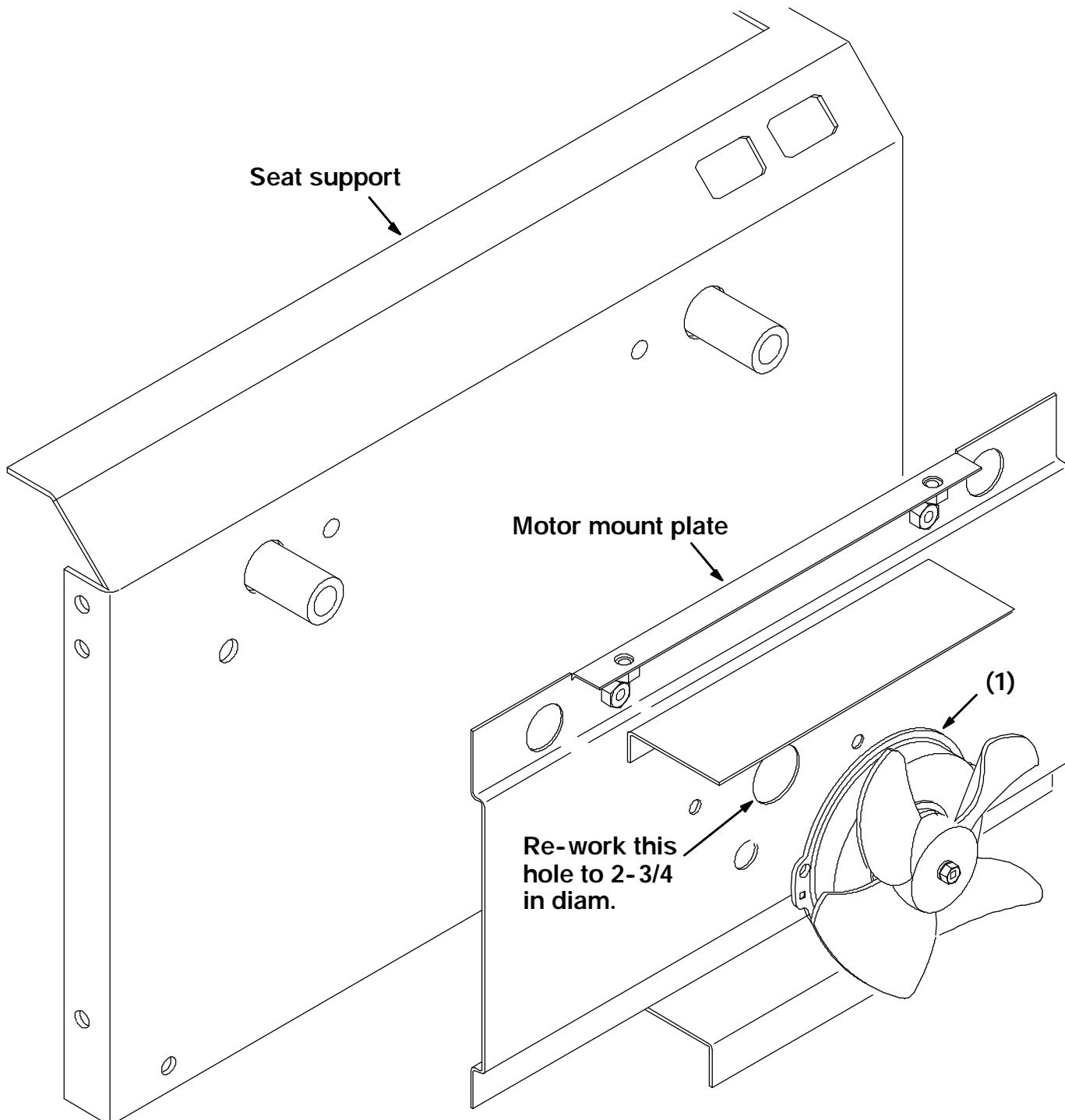
**FIG. 1 - Fan And Mount Assembly**
