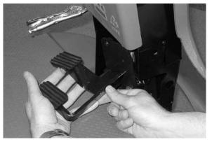
10. Using a spring puller or screwdriver, remove the 2 springs from the pedal assembly and dispose.
