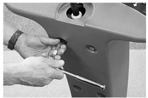
Carefully slide the rotomold housing upward about 6"/15cm to access the pedal assembly. Use vise grips to hold housing in place.
