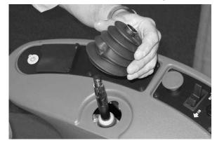
5. Remove the 4 steering column bolts using a 13mm socket wrench.
