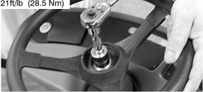
3. Remove steering wheel by tapping on spokes with rubber mallet. Be careful not to misplace the shaft key.
