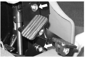
9. Remove the pedal assembly from the machine.
