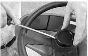
2. Remove steering wheel mounting hardware using a 19mm socket wrench.
