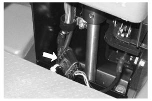
8. Remove the 2 pedal assembly mounting bolts using a 13mm wrench.
