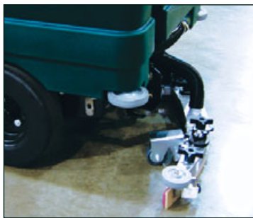
Breakaway squeegee prevents damaging walls and squeegee.
