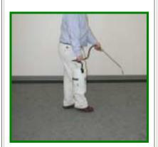
Using a recommended traffic lane pre-spray chemical, fill a pump-up sprayer with the pre-spray solution at the recommended dilution rate. Then, pressurize the sprayer and begin to apply a light coating of pre-spray chemical over the area to be cleaned; especially the entryways and high traffic patterns. Do not let the chemical dry before cleaning - try to use about a 5-10 minute dwell time. Do not cover areas that are too large.
